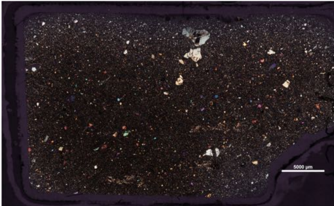
Figure 3.2: A representative thin section of the basanites. Sample is 75244, refer to Table 3.1 for a description.
