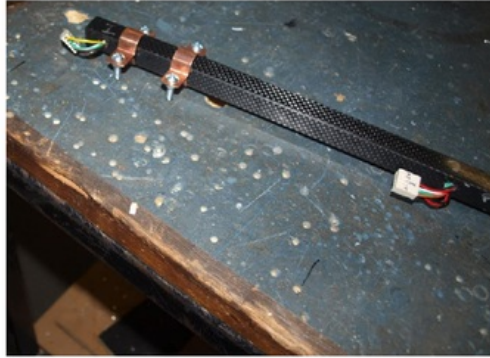
Figure 3.2: Attached Hose clamps for use of Weight system
