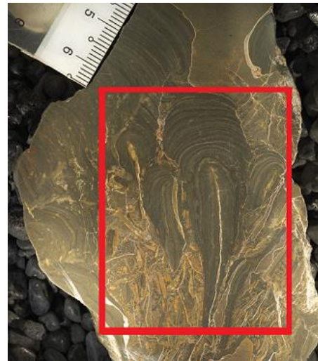
Figure 37. Hand specimen of WP1, the red box indicates the section that was element mapped with XRF.
