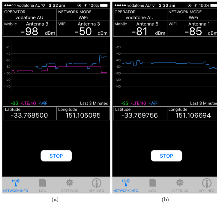
Figure 3.1: Reference Signal Received Power for a)indoor area, b)outdoor area
