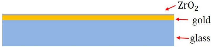
Fig. 1-5 Gold slab consisting of 30 nm gold (with a 10 nm protective layer of Zirconia) deposited on glass
