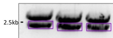
FIGURE 3.17: Digested pGEM-T_ zCCNF clones. Image of gel electrophoresed sample of digested pGEM-T_ zCCNF wild type and p.S623G mutant clones. Purple boxes indicate section of gel removed for purification of zCCNF product.
