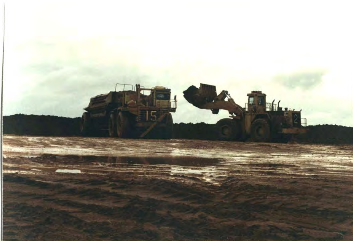
Plate 16b: A front-end loader scoops up the bauxite-rich soil and pours it into an awaiting truck's belly.
