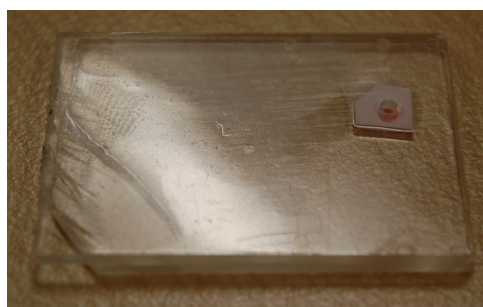
Figure 5.14: Sample containing a membrane bonded between two COC pieces
