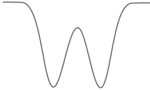
Figure 5.5: Illustration of the profiler graph showing the imperfect emboss in Method 1
