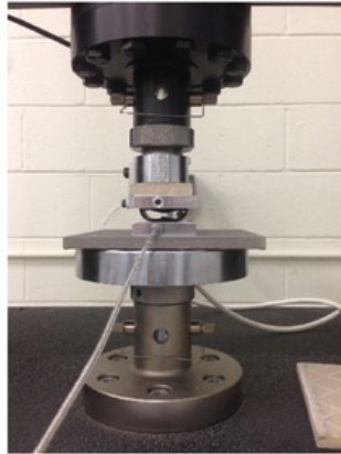
Figure 6.9: HDPE Melting in Compression
