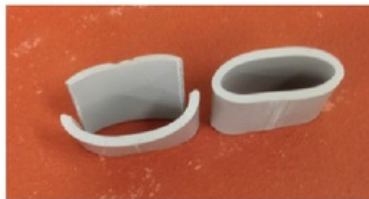
Figure 6.7: PVC Pipe Rupture
