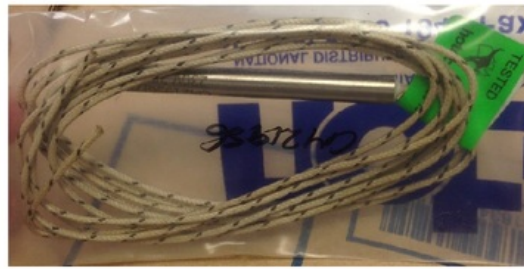
Figure 3.5: Purchased Hotco Cartridge Heater
