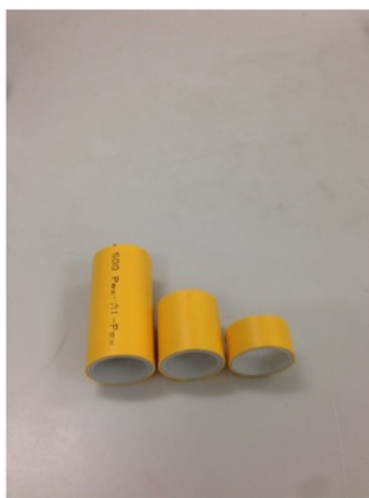
Figure B.4: PAP Pieces Prepared by METS
