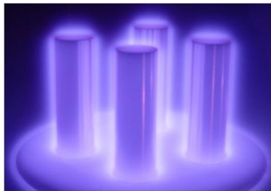
Figure 3 Example of Plasma Discharge Glow inside the PACVD Vacuum Chamber
