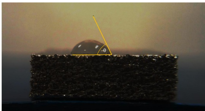
Figure 13 Example of Contact Angle Measurement of 3D-Ti64 (V) Sample using ImageJ
