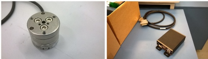
Figure 3.4: The Nano25 force torque transducer with the DAQ box
