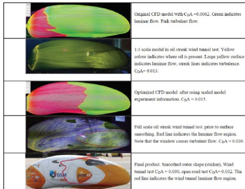
Figure 2.9: Development of the first Velox HPV shell [9].
