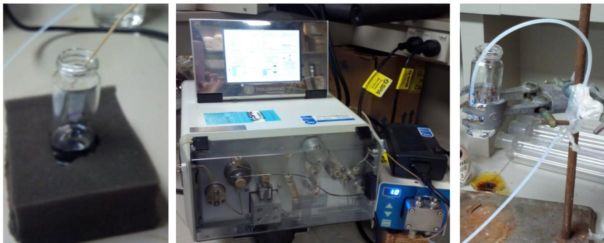
**Appendix 4: Photoreduction experimental setup using the Mercury Vapour Lamp, foil-covered H<sub>2</sub> (g) balloons and the sample reaction vials with the molecular sieves.**
