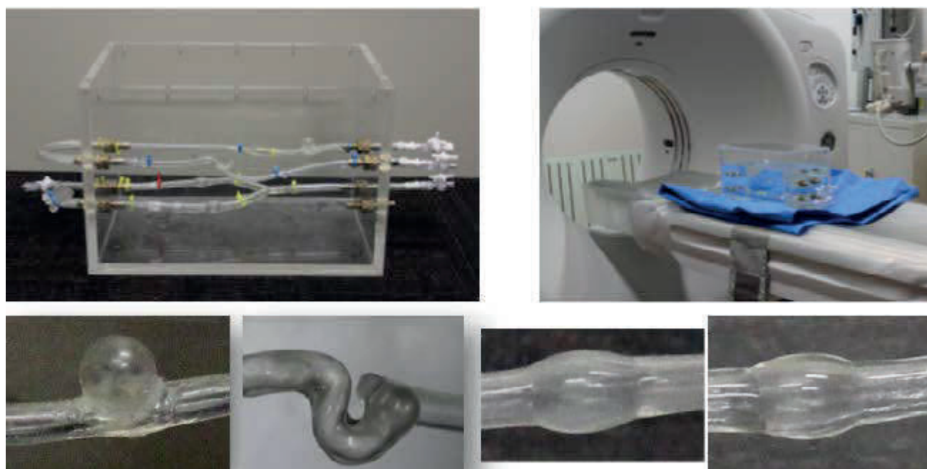
Figure 6.1: Experiment equipment. Four types of silicone aneurysm models and the CT scan. Top left: the silicone models in a plastic container. Top right: The models in the CT scan. Bottom from left to right: model 1 shift to model 4.
