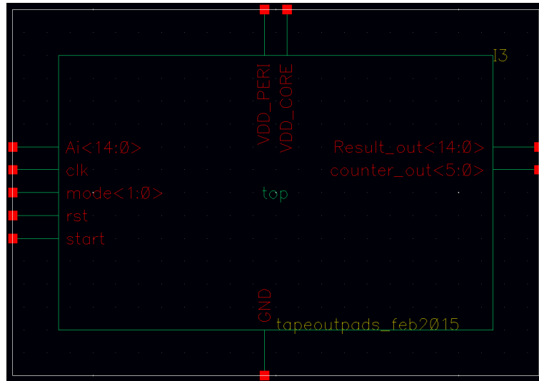
Figure 5.8: Modified symbol of top cell of modular multiplier chip
