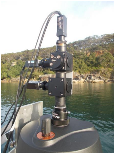
Figure 3.26 – Two-colour sensing system (as shown in in Figure 3.24a with an added excitation wavelength detection channel) mounted on a telescope receiver for field sensing experiments.
