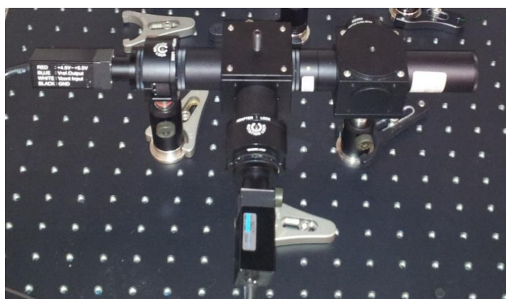
Figure 3.25 – Sensing system designed for temperature sensing with the two-colour method (as shown in Figure 3.24a).
