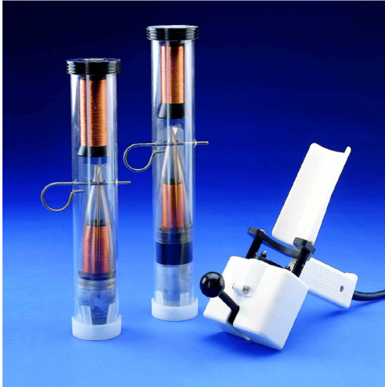
Figure 1.3. Expendable bathythermographs (probes) and hand launcher. Image acquired from [17].
