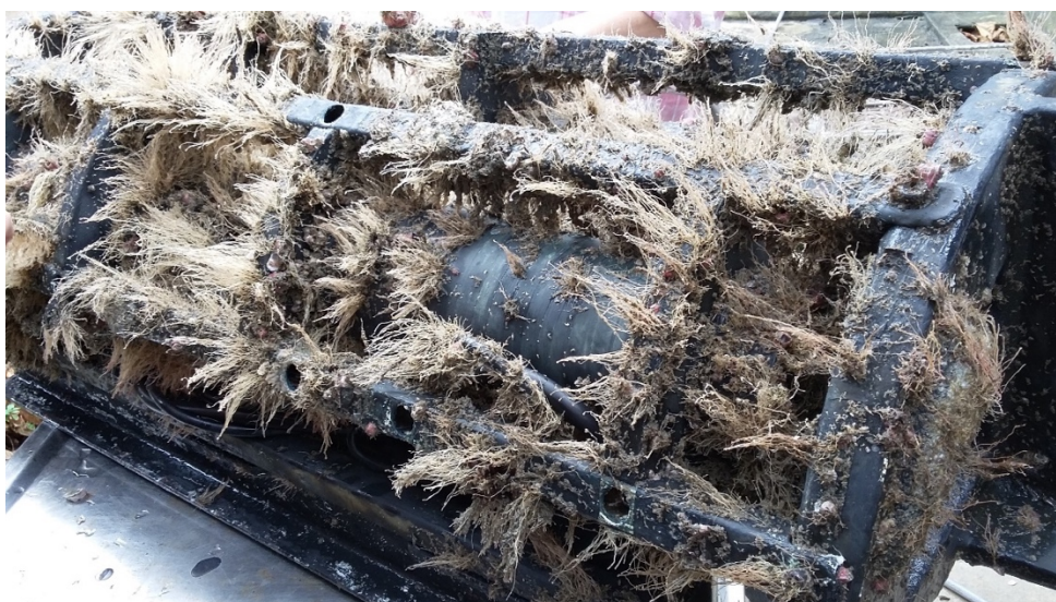
Figure 1.2. Bioincrustation accumulating inside an oceanographic buoy. Photo courtesy of Camilla Bonatto and SIMCOSTA team.
