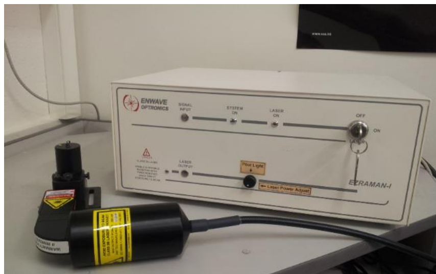
Figure 2.3. Enwave EZRaman-I spectrometer (photo from [52]).
