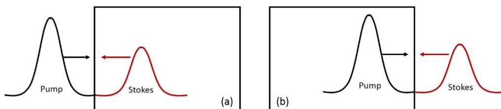
Figure 2.16 Backward Stokes pulses crossing the pump pulses at different portion of the Raman crystal.
