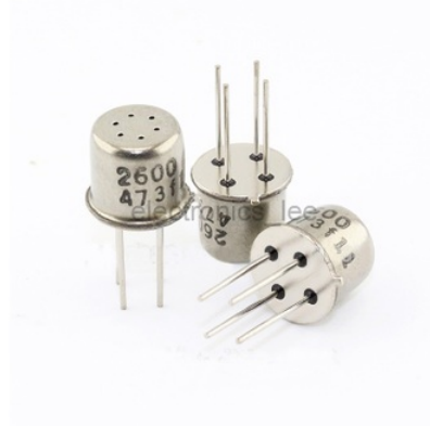
Figure 3.4: TGS2600 General Air Quality Sensor [1]
