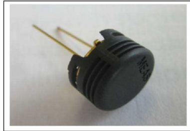
Figure 3.2: HS1101LF Relative Humidity Sensor
