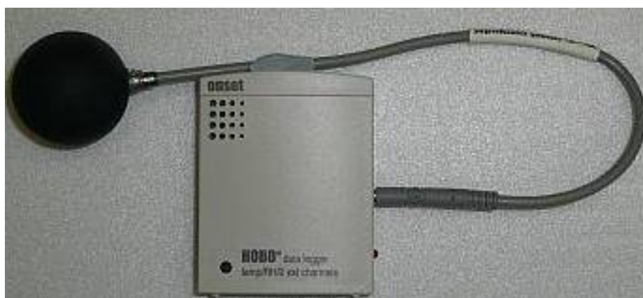
Figure 3.10: “HOBO” U12-013 Temperature and Relative Humidity Datalogger with 40mm sphere painted matte black attached to TMC1-HD Water/Soil Temperature Sensor.
