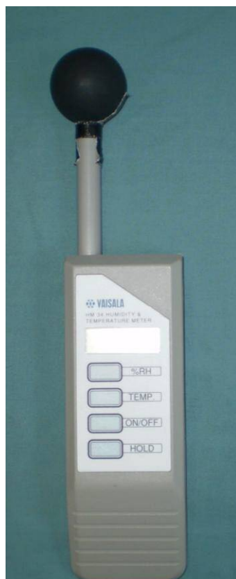
Figure 3.13: “Vaisala” HM34C Humidity and Temperature Meter with 40mm sphere painted matte black.
