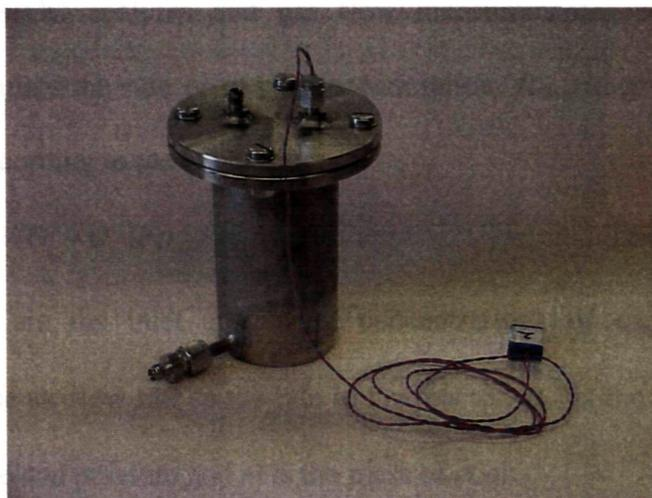
**Figure 2.3.** One of the reactors used for the oxidation rate measurements. Air entered at the bottom fitting and exited at the top. The thermocouple for monitoring the sample temperature is visible.
