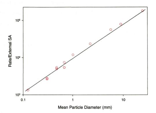
Figure 3.15. Oxidation rate at 90 °C normalised to the spherical external surface area
