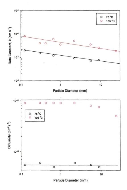
Figure 4.14. The dependence of the values estimated for the rate constant (a) and diffusivity (b) on particle size using the modified shrinking core model
