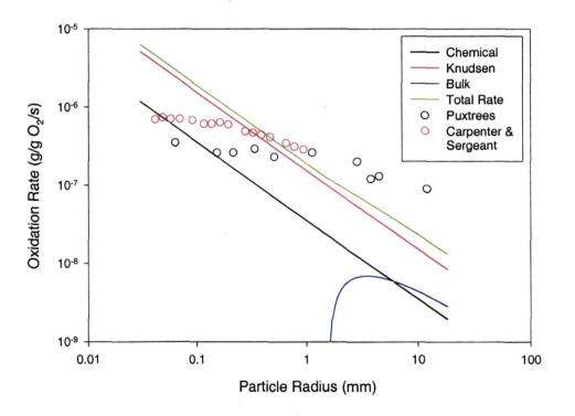
Figure 4.16. Oxidation rates predicted by the pore tree model for the chemical kinetics, Knudsen diffusion, bulk diffusion and overall rate using the parameters listed in Table 4.2. The data for Puxtrees coal were measured at t = 0 days at 105 °C.
