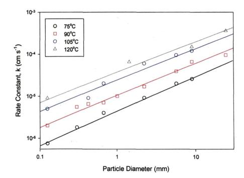
Figure 4.10. The dependence of the values estimated for the rate constant, k, on particle size
