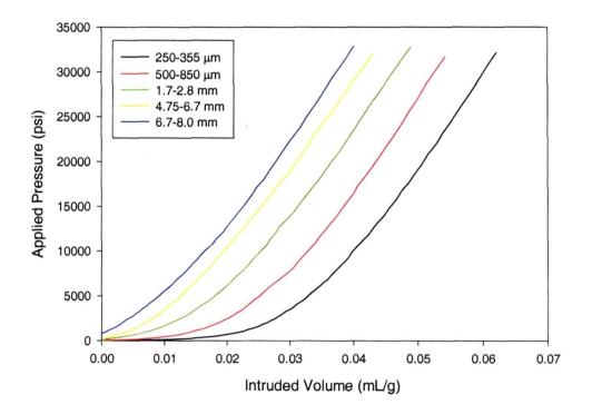
Figure 3.4. Mercury porosimetry pressure - intruded volume curves for various particles size fractions
