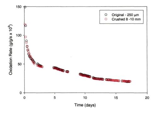
Figure 3.11. Comparison of oxidation rate curves for 8-10 mm which had been crushed to -250  $\mu m$  and the original -250  $\mu m$  fraction
