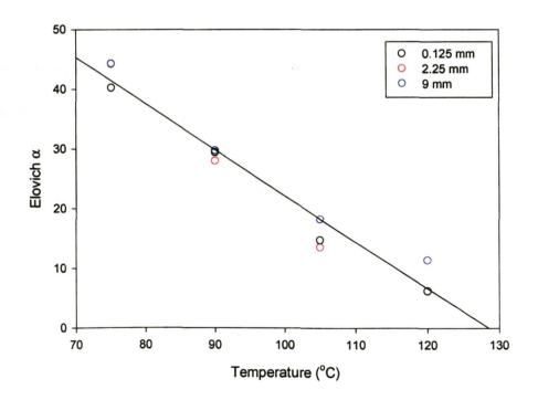
Figure 4.5. The dependence of the Elovich  $\alpha$  parameter temperature
