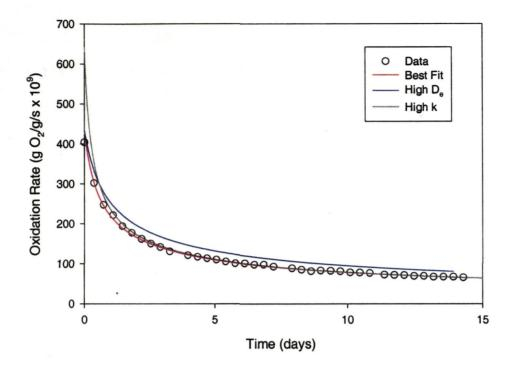
Figure 4.8. Comparison of experimental results for 1.44 mm particles at 120 °C with the SCM calculated curve. The effect of varying k and  $D_e$  is also shown – best  $k = 6.50 \times 10^{-5}$  cm s<sup>-1</sup>, high  $k = 9.75 \times 10^{-5}$  cm s<sup>-1</sup>; best  $D_e = 1.50 \times 10^{-9}$  cm<sup>2</sup> s<sup>-1</sup>, high  $D_e = 2.25 \times 10^{-9}$  cm<sup>2</sup> s<sup>-1</sup>
