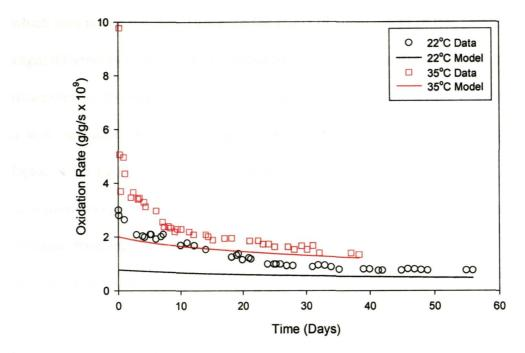
Figure 4.6 Comparison of measured oxidation rates at 22 and 35 °C to those predicted by the Elovich model
