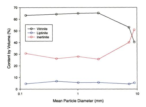
Figure 3.2. The dependence of petrographic composition of Puxtrees coal on particle size
