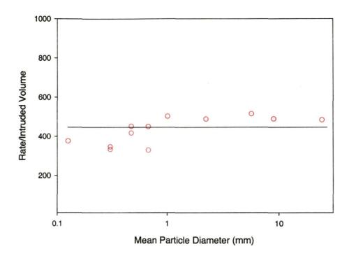
Figure 3.16. Oxidation rate at 90 °C normalised to the mercury intruded volume
