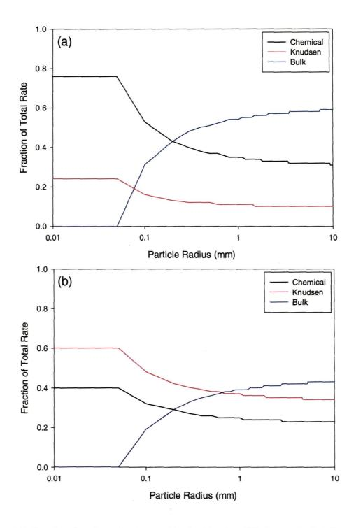
Figure 4.15. Fraction of total rate for chemical kinetics, Knudsen diffusion and bulk diffusion. (a)  $k = 4 \times 10^{-7}$ ; (b)  $k = 4 \times 10^{-6}$  cm s<sup>-1</sup>
