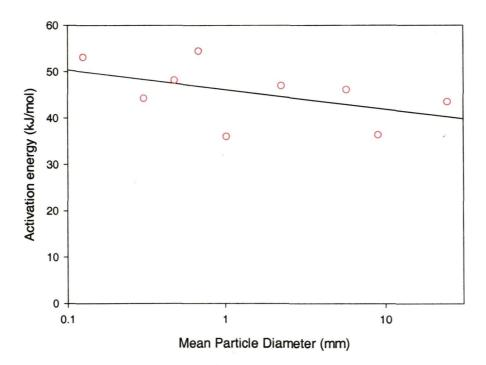
Figure 3.10. The dependence of apparent activation energy on particle size
