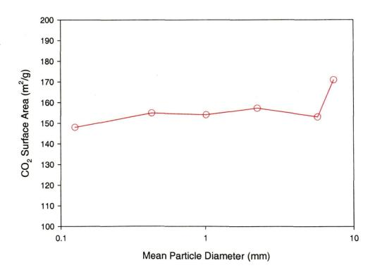
Figure 3.6. The dependence of CO<sub>2</sub> surface area on particle size
