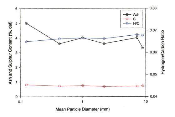
Figure 3.1. The dependence of chemical composition on particle size
