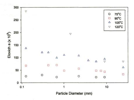
Figure 4.4. The dependence of the Elovich *a* parameter on particle size
