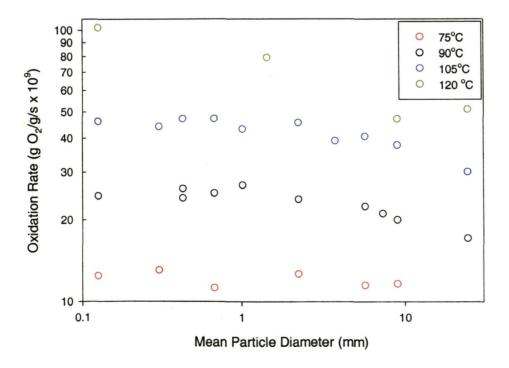
Figure 3.14. The dependence of oxidation rate (measured at 10 days) on particle size
