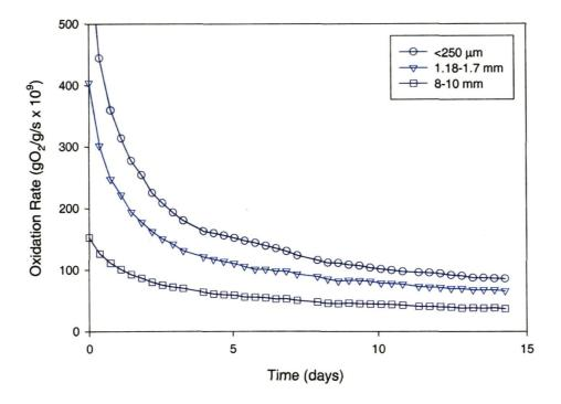
Figure 3.12. The dependence of oxidation rate (at 120 °C) on particle size
