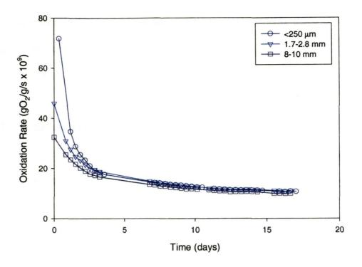
Figure 3.13. The dependence of oxidation rate (at 75 °C) on particle size
