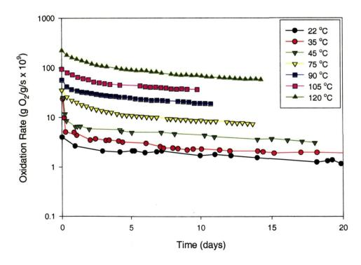
Figure 3.8. Oxidation rate as a function of time for the full range material at temperatures from 22 to  $120\ ^{\circ}\mathrm{C}$
