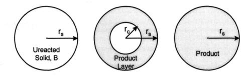
Figure 4.7. Progress of reaction in the shrinking core model (from Denbigh and Turner, 1971)
