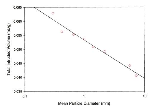
Figure 3.3. The dependence of total intruded volume on particle size
