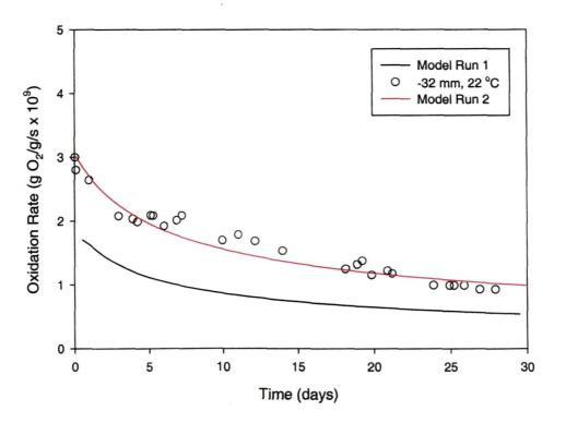
Figure 4.11. Comparison of measured rate data with rates calculated with the shrinking core model
