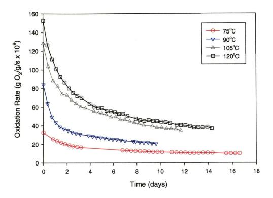
Figure 3.7. Oxidation rate as a function of time for 8-10 mm particles of Puxtrees coal
