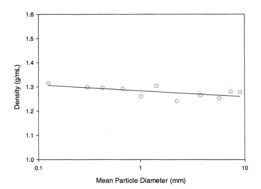
Figure 3.5. The dependence of helium density on particle size
