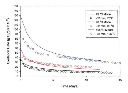
Figure 4.12. Comparison of measured data for 75, 90 and 105 °C with rates calculated with the shrinking core model
