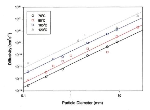
Figure 4.9. The dependence of the values estimated for the diffusivity,  $D_e$ , on particle size
