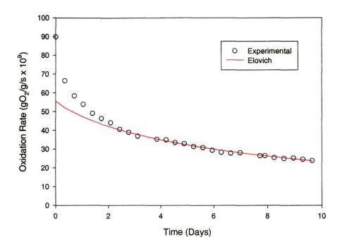
Figure 4.3. Comparison of Elovich model with experimental data for Puxtrees coal at 90 °C. The particle size was 1.7-2.8 mm.
