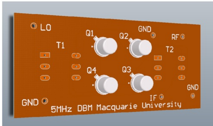
Figure 4.7: 3D representation of the mixer in CircuitMaker.
