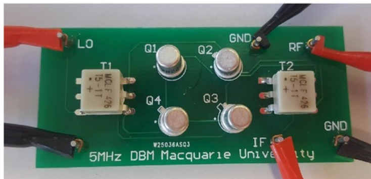
Figure 4.8: Mixer under test with the PCB containing soldered components.
