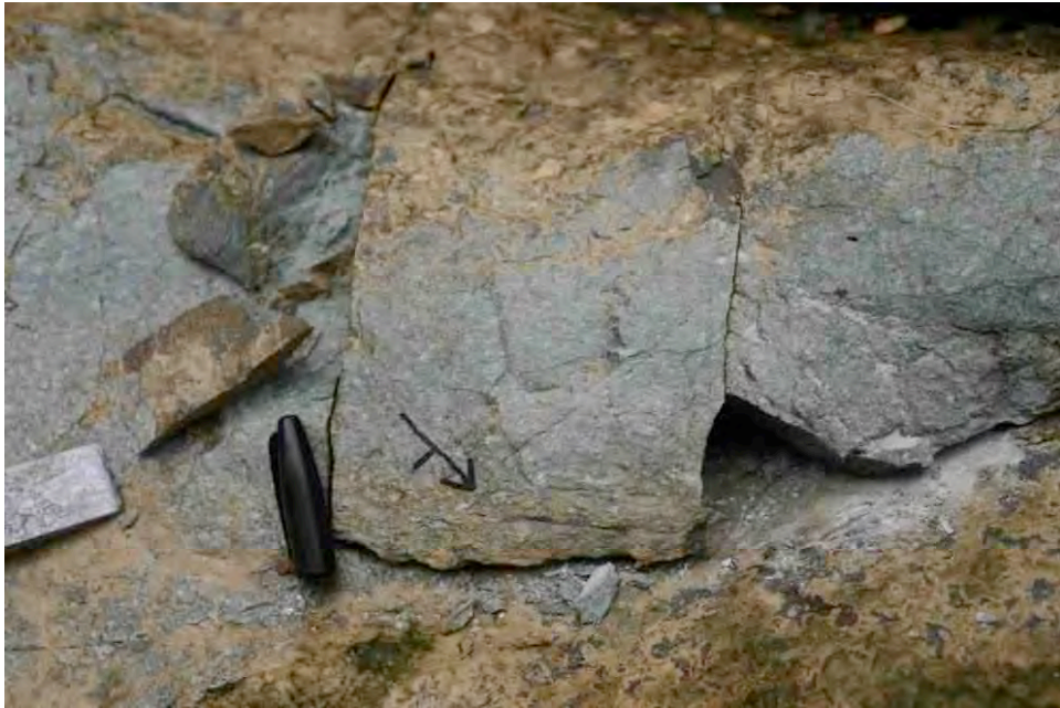
Figure 3.2 Orientation of a flat face of a rock sample, Ampae Ck. Measurement is of a foliation plane in metabasite.
