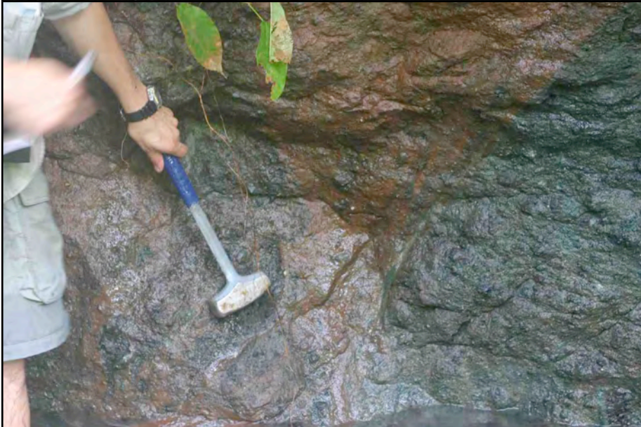
Figure 5.36 View looking W of an oxidised brittle fault zone, Dare Creek. The long handle crack hammer is 400 mm long.
