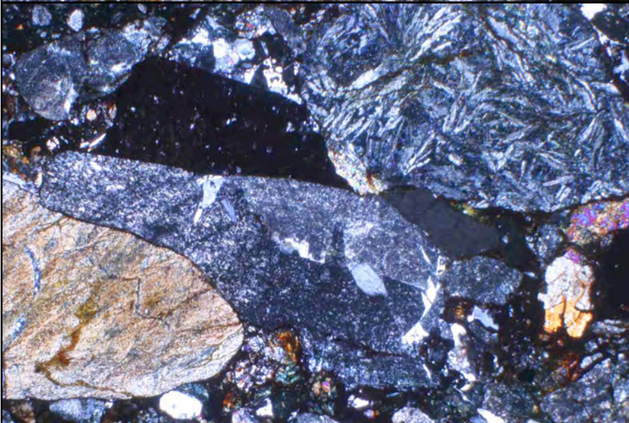
Figure 4.14 Photomicrograph showing blastodoleritic to blastobasaltic texture in upper right and middle clasts, sample 0607, Dare Creek. Field of view is 3.5 mm across.
