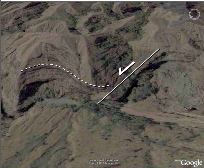
Figure 5.34 Google Earth™ image view looking SE of the Gwoira Conglomerate. A normal fault is marked by a solid line. S0 is marked by a dashed line.
