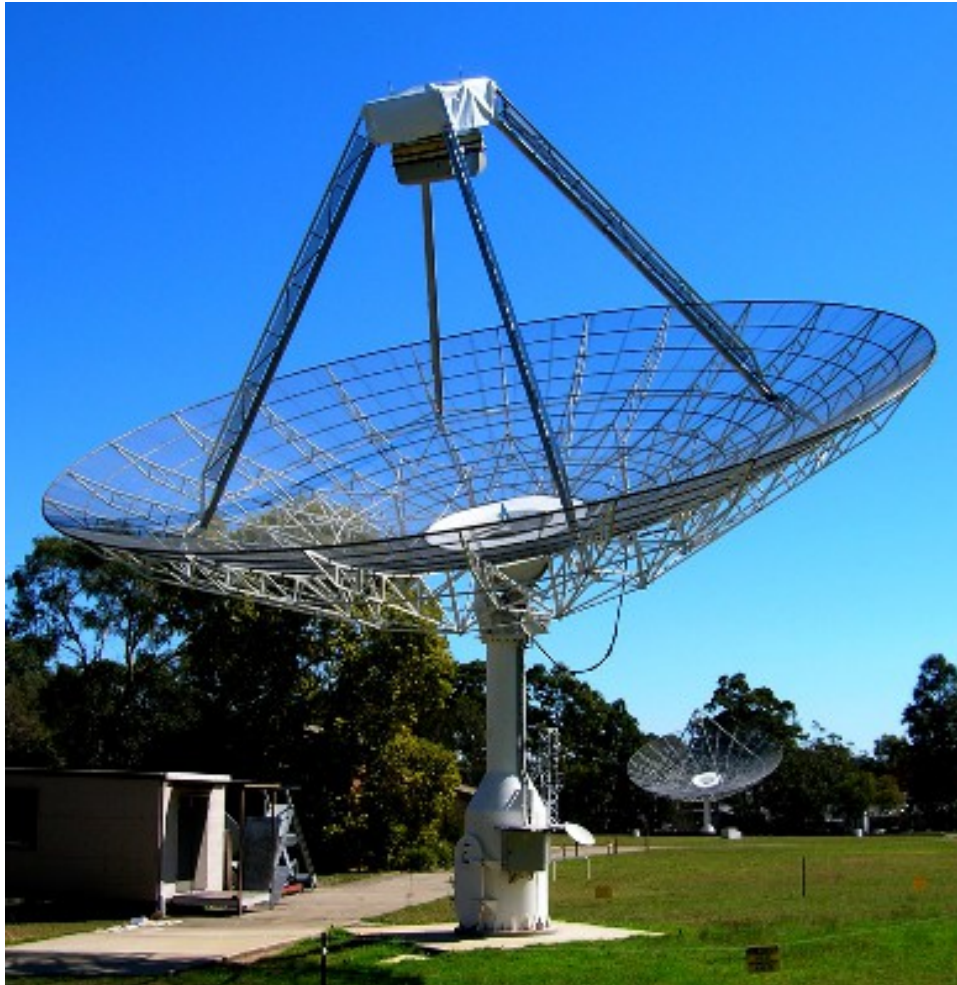
Figure 6.1 – The two-dish prototype radiotelescope located in Sydney; the east antenna in the foreground is fitted with the FPA and the west antenna in the background with a single horn.
