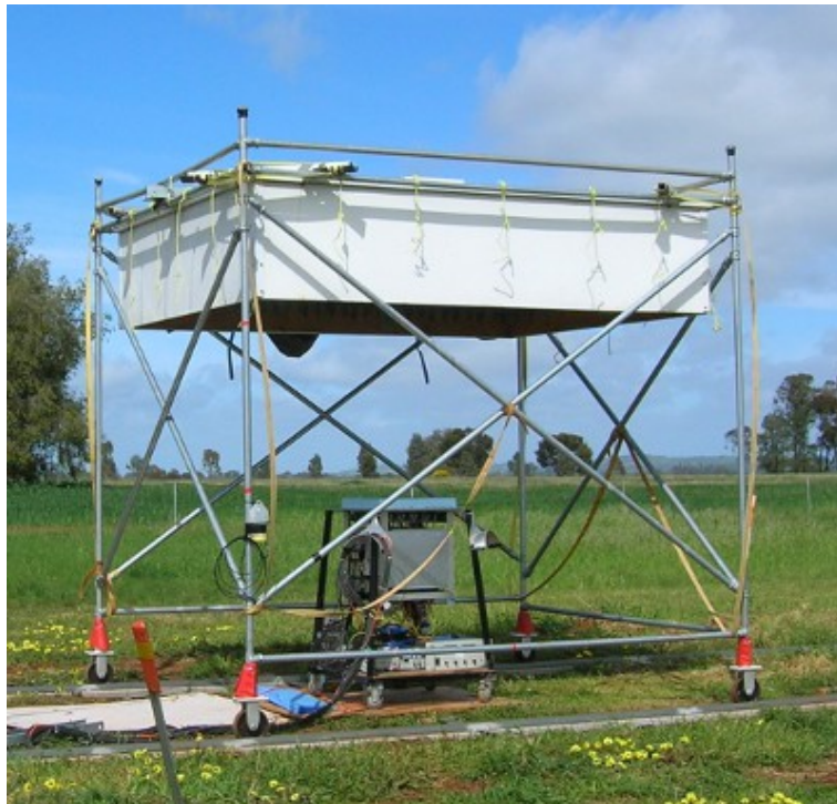
Figure 9.2 – Y-factor Measurement of a prototype FPA. The absorber sheet is mounted in the box above the array. The hot load can be wheeled off the array for the cold-sky measurement. The array under test is a prototype for the ASKAP project.
