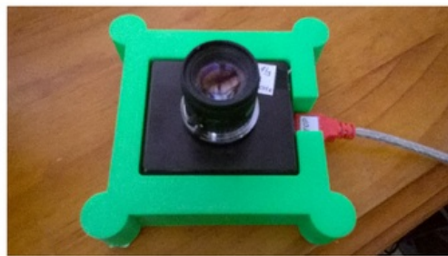
Figure A.3: Bottom camera mount with the mounted camera.
