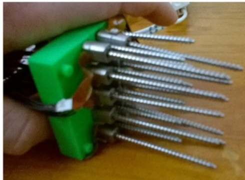
Figure A.6: 20 mounted motors (some lead screws are loose due to the heat of operation melting the surrounding plastic).
