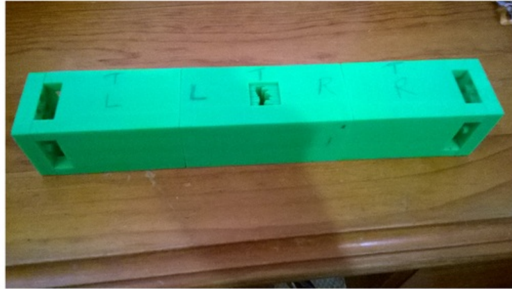
Figure 4.1: The five assembled sections of the MLC housing with the leaves also in place.
