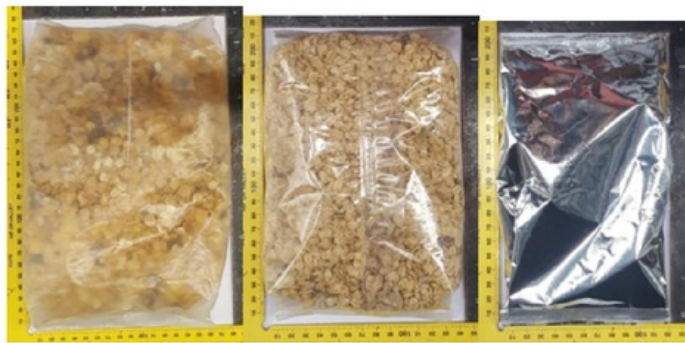
Figure 4.6: (left) Bag Opaque Bag 180 mm x 280 mm, (middle) Bag Clear 145 mm x 215 mm, (Right) Bag Foil 120 mm x 208 mm
