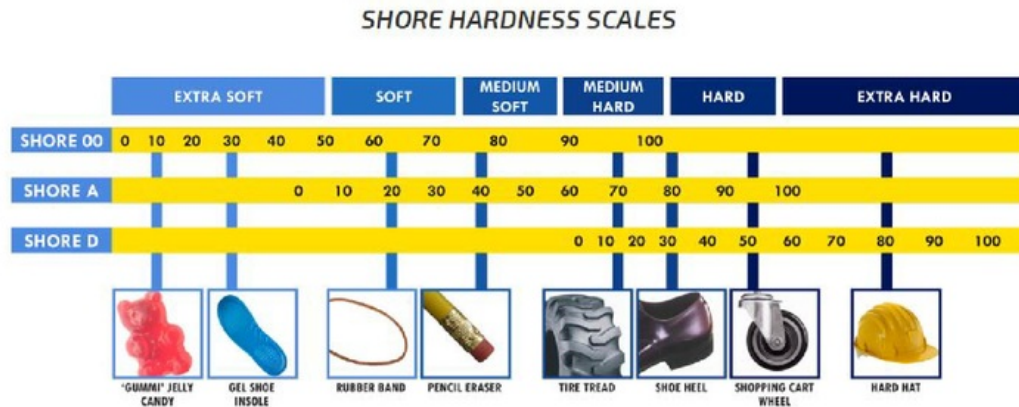
Figure 2.13: Shored hardness scale types converted between each type [20].
