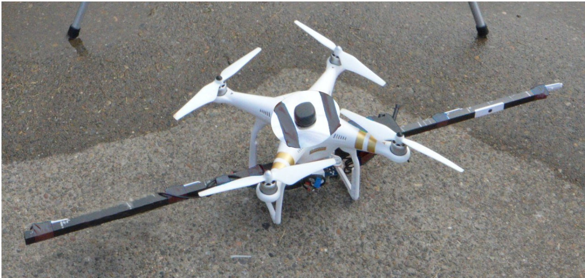
Figure 16 - Magnetic Gradiometer Array on board the DJI Phantom Pro 3. The circular ground plane, centre, was required to be smaller for propeller clearance on the DJI, at 8cm diameter.
