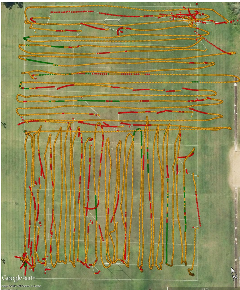
Figure 33 (Left) - Flight tracks using field based DGPS as recorded during flight. Green dots indicate Fix, Yellow Float, and Red Single mode positioning. Despite using a complete RTK differential GPS system, there are many deviations and DGPS drop outs during flights. This is hoped to be corrected with the Kalman filter
