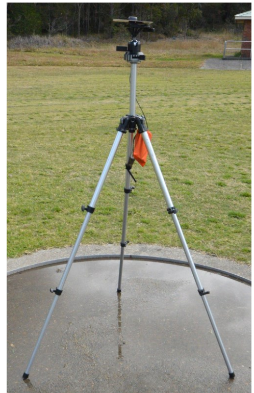
Figure 23 - Reach local base station above survey mark. The base station was moved to the central field during later tests due to poor sky view at this location.
