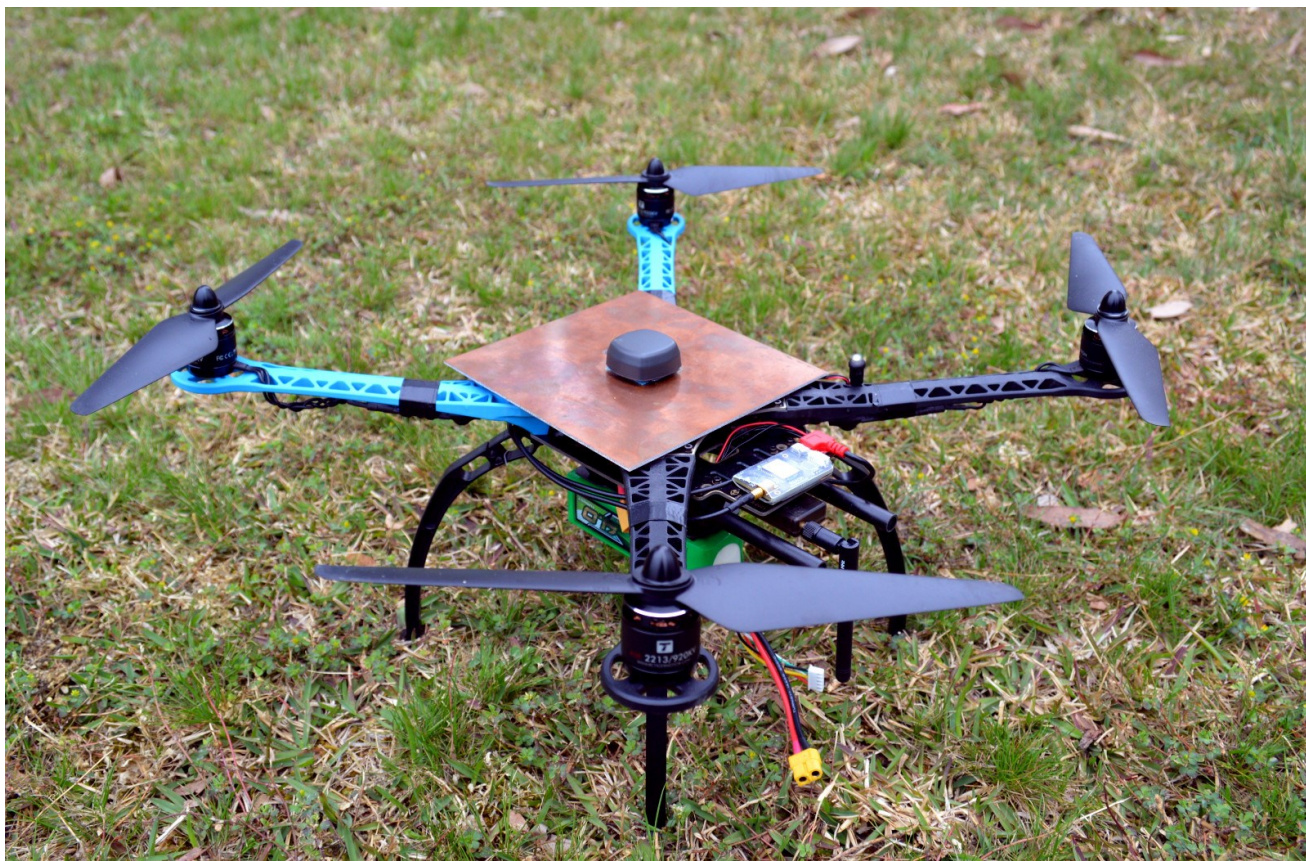
Figure 17 - Custom UAV with Reach GPS module present. The copper groundplane (15x15cm) is prominently featured beneath the GPS antenna in the centre image, and blocks electric interference from the flight control system. The Reach GPS can be used for UAV navigation as well as data sample positioning. The magnetic gradiometer system mounts easily to two service rails running the length of the frame, or could be attached to a suspended gimbal.
