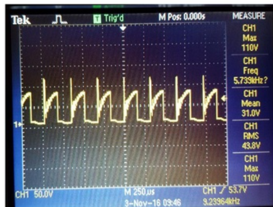
FIGURE 19 TYPICAL WAVEFORM ACROSS PRIMARY. TRANSIENT RESPONSE INCLUSIVE OF INDUCTIVE SPIKE
