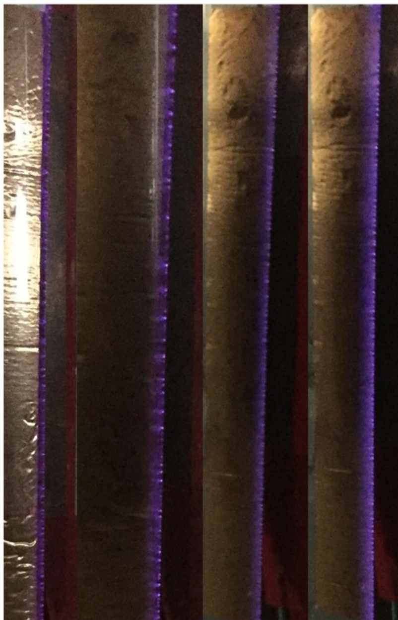
FIGURE 25 DBD PLASMA FORMATIONS, (LEFT) FROM LEAST (1) TO MOST (4) BRIGHTEST. NOTICE THE DENSITY OF THE PLASMA DISCHARGES ACROSS THE ELCTRODES.
