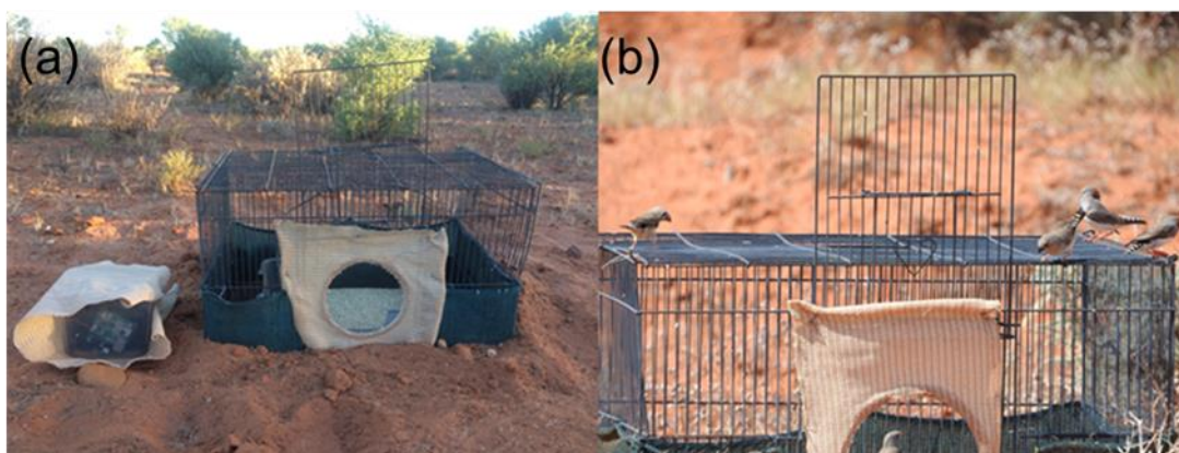
Figure 3 Artificial feeders equipped with seeds in the tray and a round antenna at the entrance connected to an RFID-decoder placed next to the feeder (a). Small flock of zebra finches, composed of males, females and juveniles (with black bill) foraging in the feeder (b).
