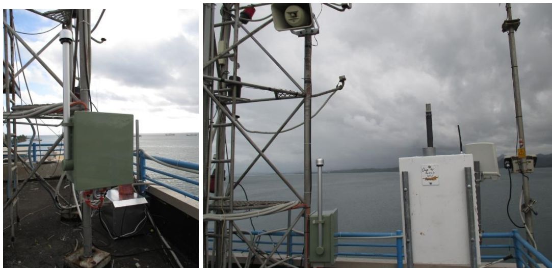
Suva City. An ASP sampler (green) is affixed to the tower that also houses Australian Bureau of Meteorology instruments. An Osiris sampler (white) is affixed on poles adjacent to the tower.
