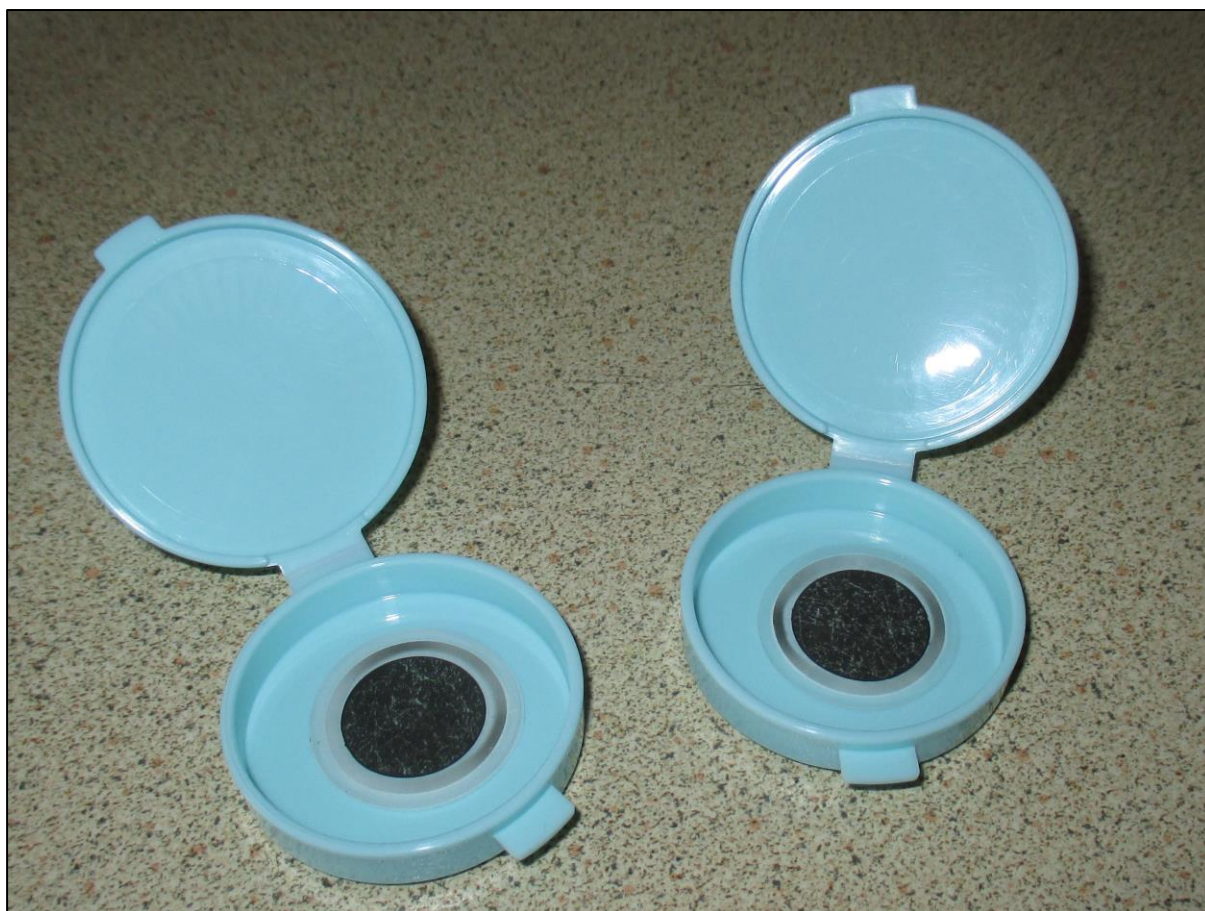
Figure 2.5 Filter samples from Suva city. The air filters each represent 24-hours sampling (30 m 3 air) and show dark-coloured particles, which were found to have a high black carbon content (Paper One). Shadowing effects evident on filter rims of these early samples (October 2014) were corrected for continued sampling.
