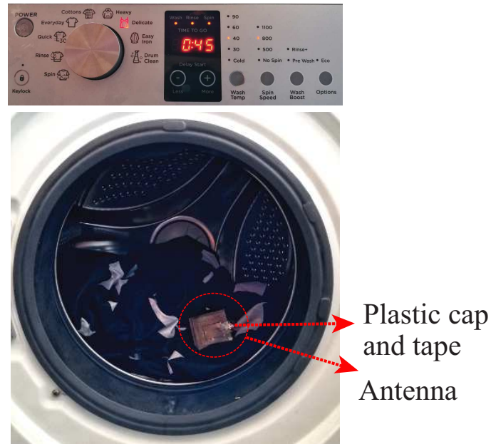
Figure 5.16: The antenna inside the washing machine.
