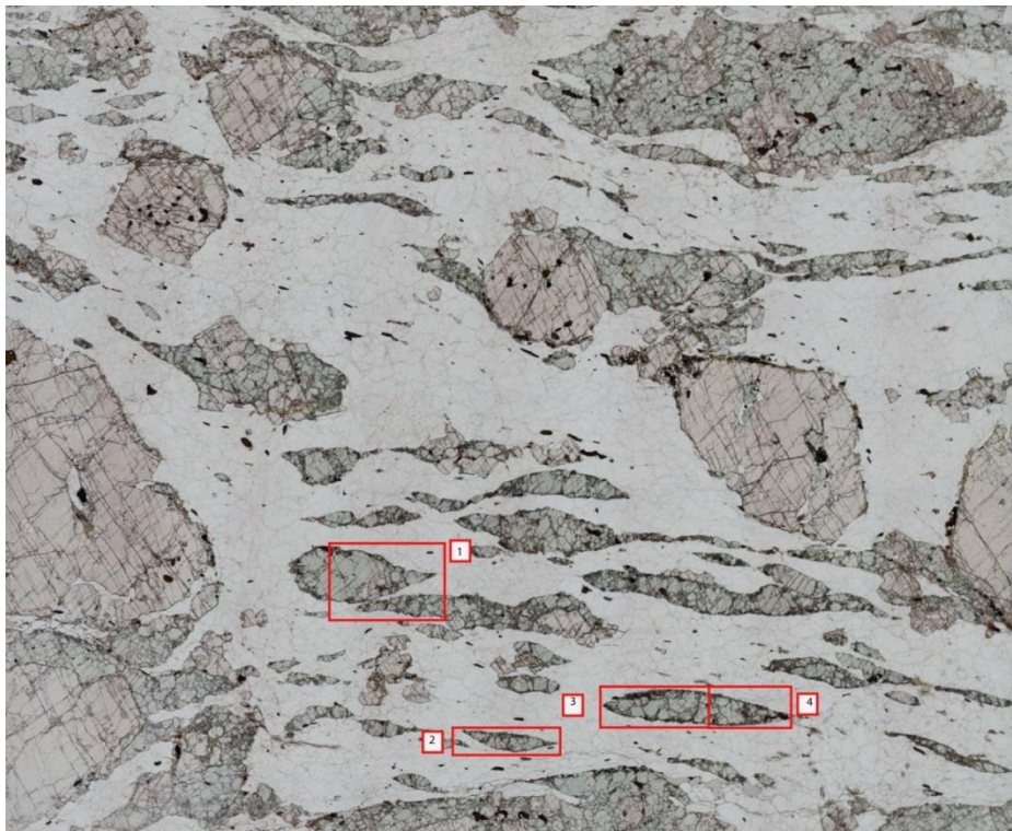
Figure 4.7 1202: Low strain OG, red boxes indicate EBSD map locations. field of view is 50mm
