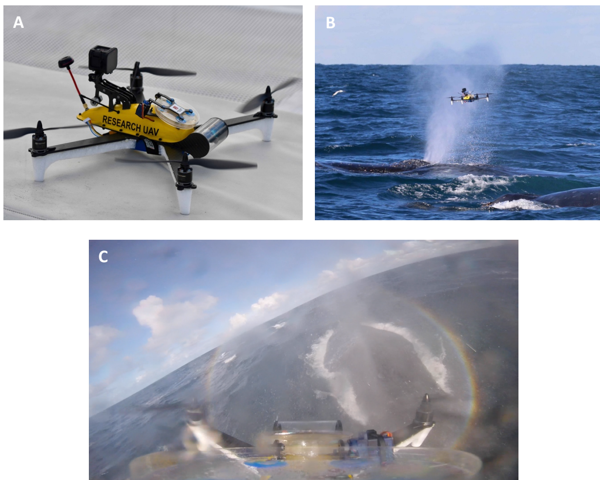
Figure 5.2. (A) Purpose-built UAV designed to sample whale blow. The UAV consists of a sandwich style carbon fibre body. White foam floats support the UAV during take-off and landings and provide floatation in water. The yellow shell houses all electrical equipment. A GoPro® hero session is mounted at the back of the yellow shell to record flights. A hinge mechanism with disposable petri dish is located in the centre of the yellow shell. This can be remotely operated to minimize sample contamination in the field. The clear round tube at the front of the UAV houses the first-person camera to assist with sampling. (B) UAV sampling whale blow. This photo was taken just as the UAV had passed through the visible blow (plume of spray). The petri dish is still in the open position. Sample was collected on both the lid and bottom (nutrient agar filled) side. The petri dish was shut immediately after collection to minimize sample contamination and the drone was flown back to the research vessel >200 meters away. (C) Screenshot from the UAVs on-board GoPro® camera mid whale sample collection. This footage shows the petri dish at the bottom of the picture. The whale is located on the right-hand side. The petri dish is completely extended (open) with blow droplets visible on both sides of the dish and GoPro® lens.
