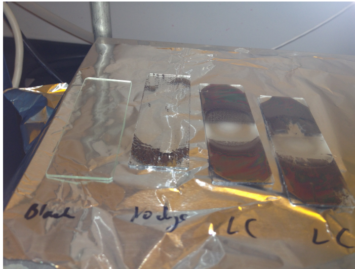
Figure 5.16: Damage to the underlying gold layer as a result of PMMA deposition. From the left, slide 2 to 4 were completely covered in gold prior to PMMA deposition. After the PMMA deposition, the gold on slide 2 is almost completely peeled off, and cracking is evident. Partial destruction of the gold film is seen in slide 3 and 4.
