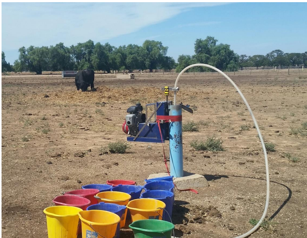
Figure 2.2 Site photo demonstrating the setup of the inertia pump for groundwater extraction and sample collection from a bore in the Murray River catchment.
