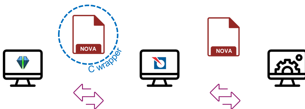
Figure 4.2: Flow of instrument commands. Control commands, themselves generated by Qudi, for the NT-MDT piezoelectric stage, written in Nova Power Script, were required first to be passed through to the Nova Px software in C.
