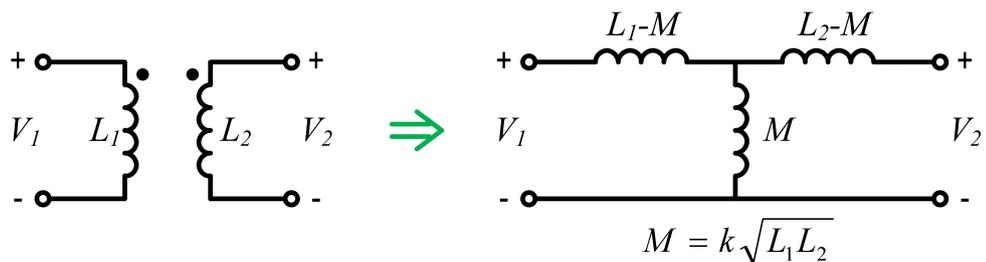
**Figure 2.6:** T model for a transformer [38].
