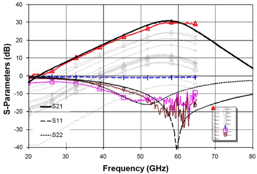
Figure 5.29: GTC2 PA measured vs simulated plots (apologies for the poor graph).
