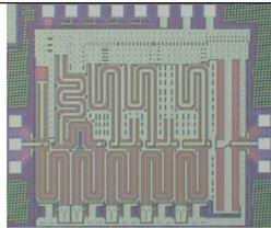
60 GHz 0.18 μm SiGe transmission line based PA, used in GTC2-TX. Manufactured by Jazz Semiconductor.
