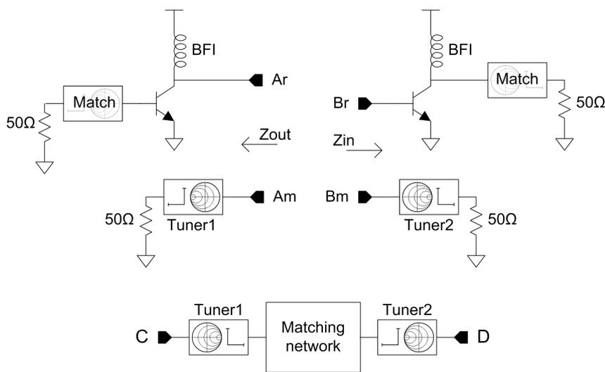
**Figure 5.23:** A method proposed for matching high power devices.
