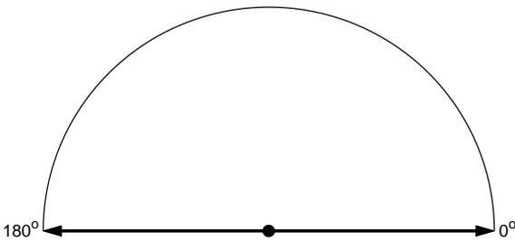
Figure 3.20: 1 element array factor
