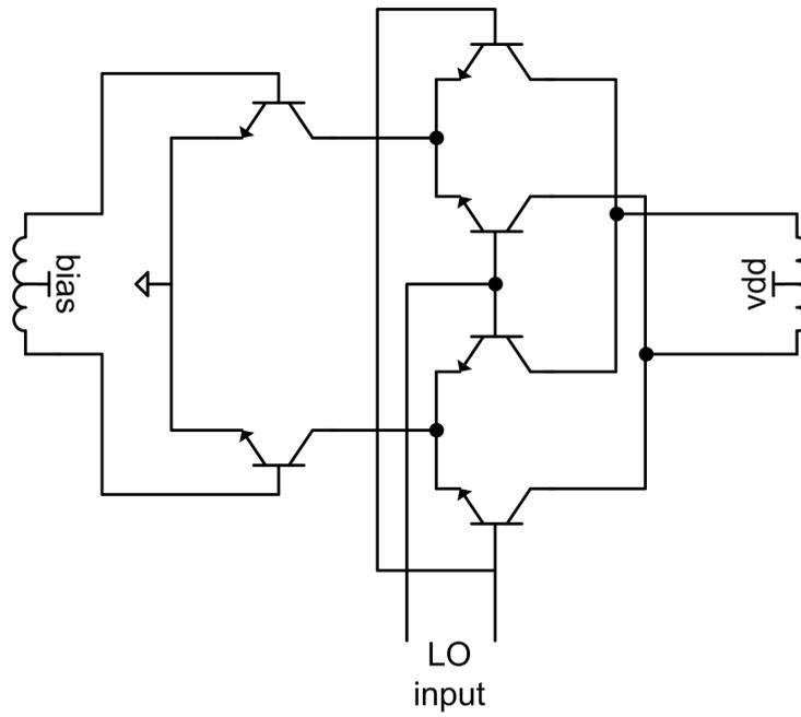
Figure 7.33: Schematic of IF to RF mixer
