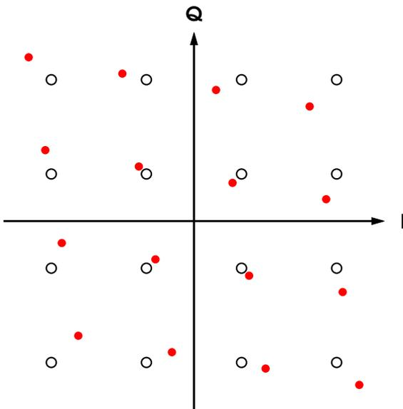
**Figure 3.7:** 16-QAM constellation with 20 degrees phase imbalance in I/Q paths.
