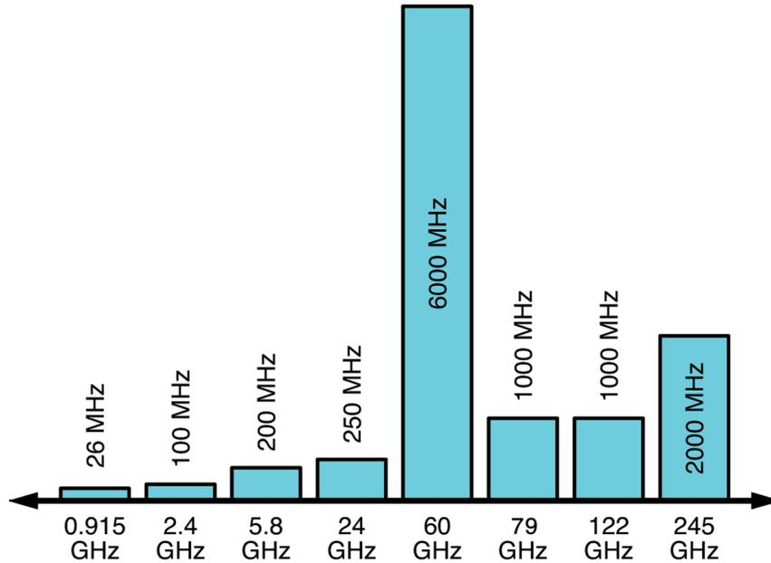
Figure 1.5: Unlicensed channel bandwidths.
