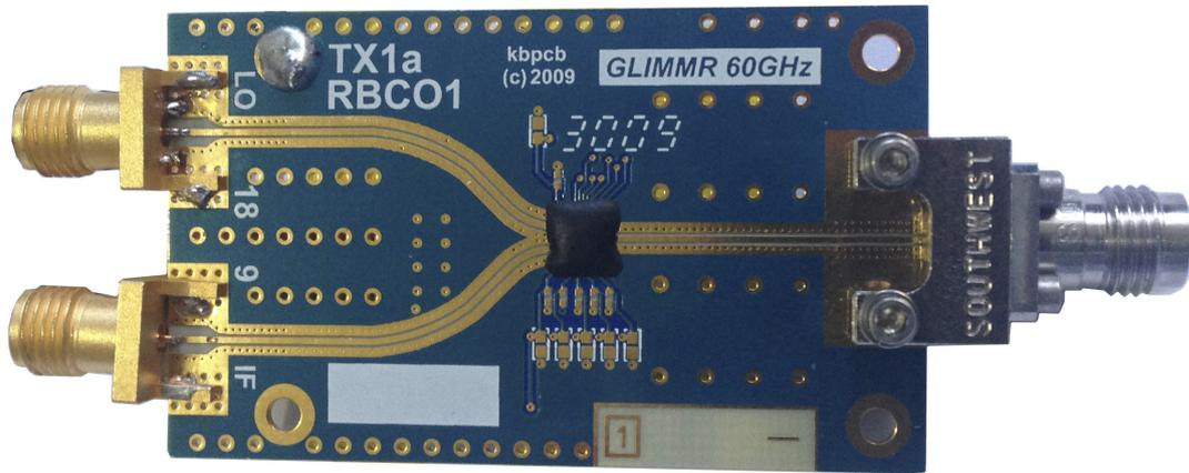
**Figure 7.38:** Photo of GTC3 module showing the die with encapsulation and the connectors.
