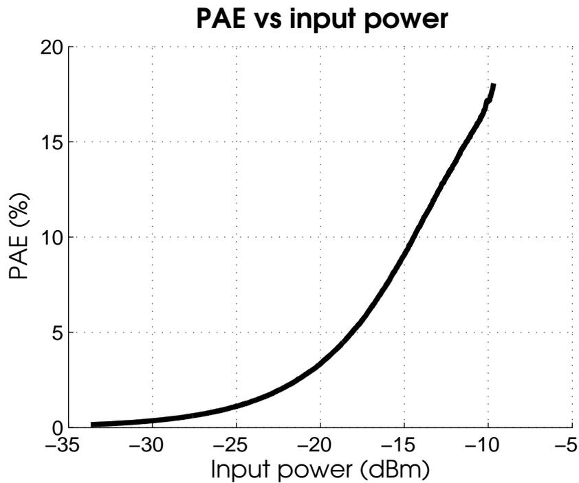
Figure 6.19: PAE vs. input power.
