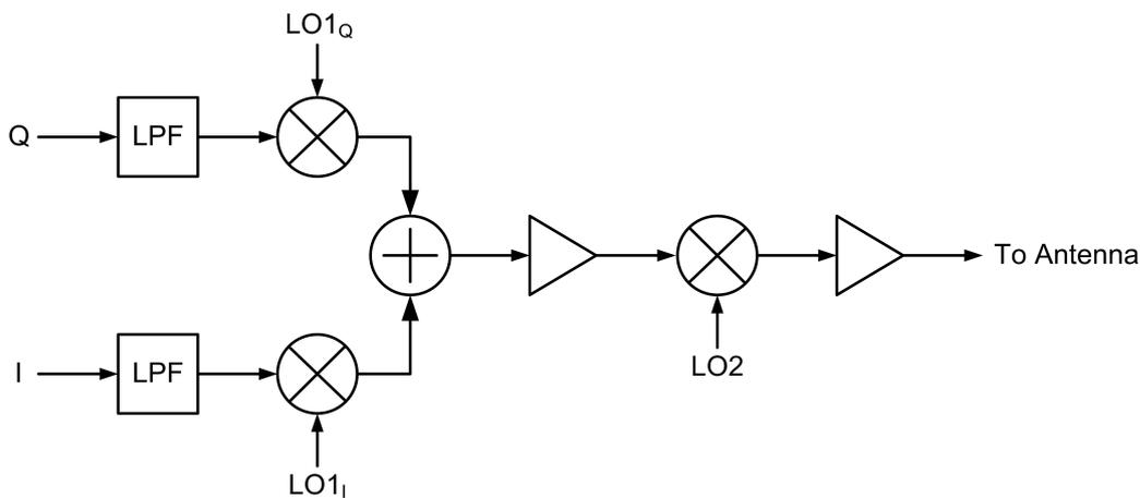
**Figure 3.4:** Dual conversion transmitter.
