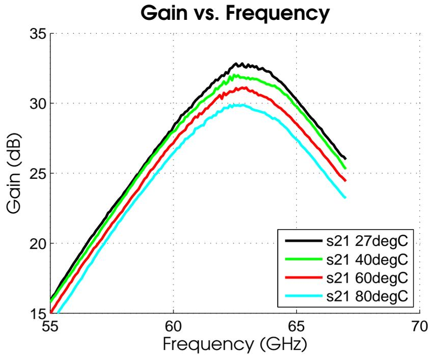
Figure 6.16: Gain (S21) vs. frequency.
