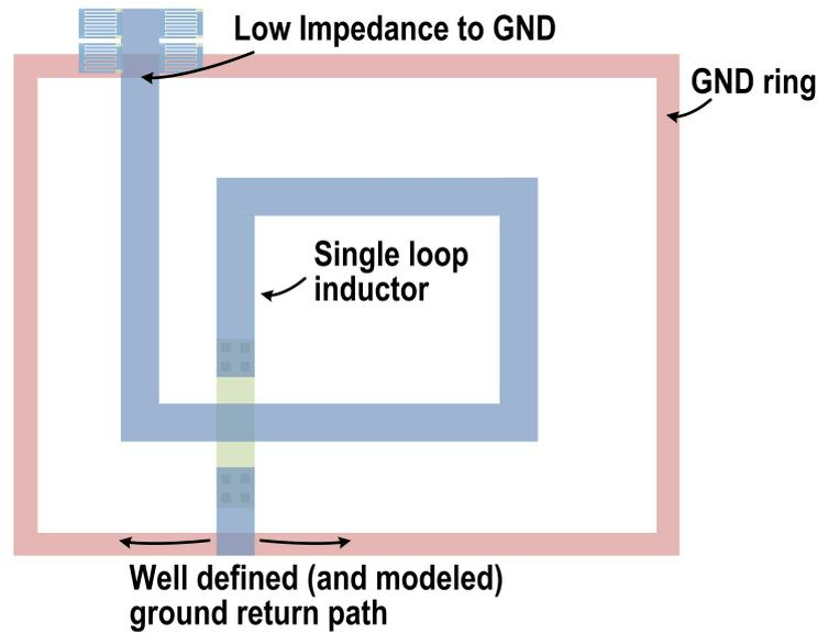
**Figure 2.5:** Inductor showing main loop, ground ring and decoupling capacitors.
