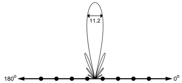
**Figure 3.23:** 8 element linear array factor,  $\frac{\lambda}{2}$  spacing
