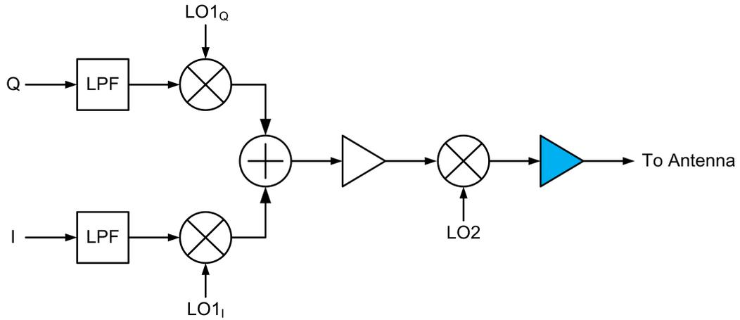
**Figure 5.1:** Block diagram of a dual-conversion transmitter with the PA highlighted in blue.
