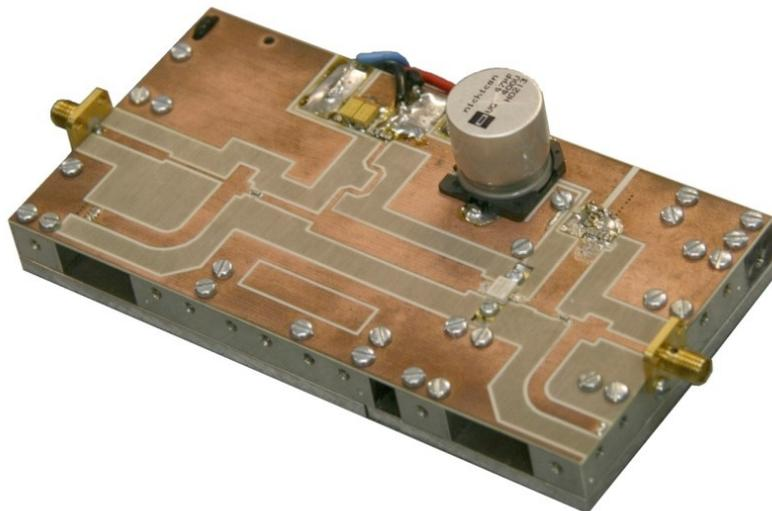
**Figure 5.21:** Photo of the finished amplifier. The board is implemented using a Rogers substrate.
