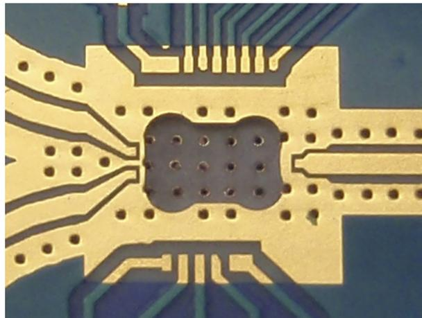
**Figure 7.39:** Photo of GTC3 module showing zoom in on the cavity for the chip.
