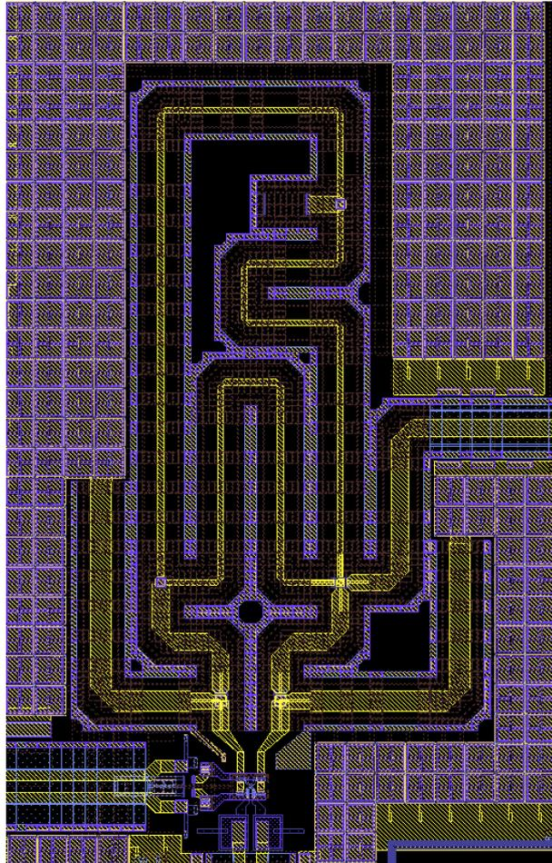
**Figure 7.10:** *Layout of the RF mixer. The output balun is a transmission line design implemented by Leonard Hall.*
