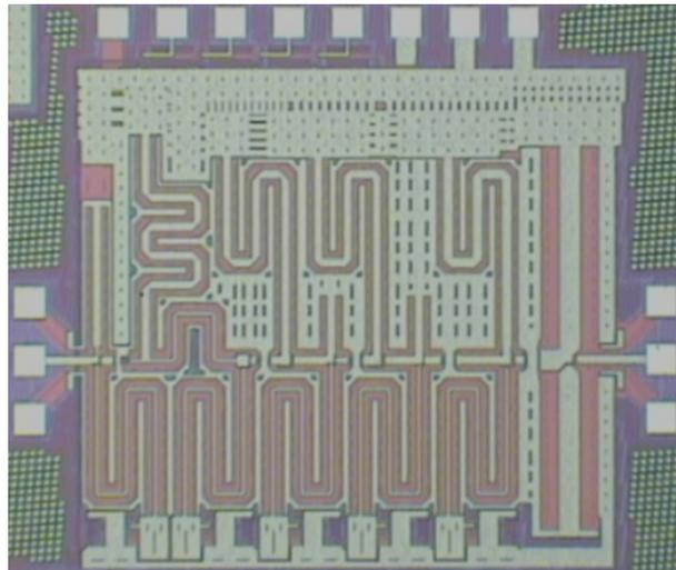
**Figure 5.30:** Die photo of the implemented PA. Die size is approximately  $1\text{mm} \times 1\text{mm}$ .
