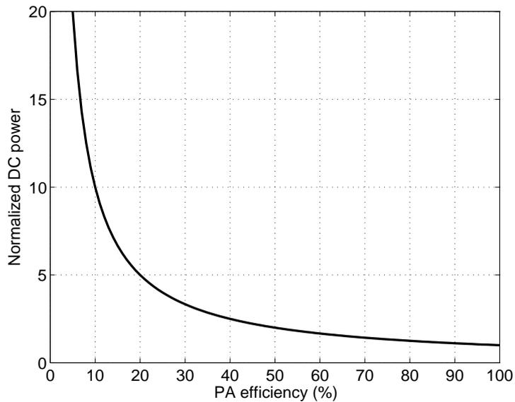
**Figure 5.3:** *Normalised DC power of a PA versus the efficiency.*
