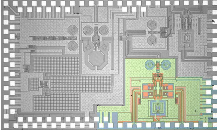
**Figure 7.36:** Chip micro-graph for Baseband to IF Chip, the TX is coloured, the rest of the chip is black and white.
