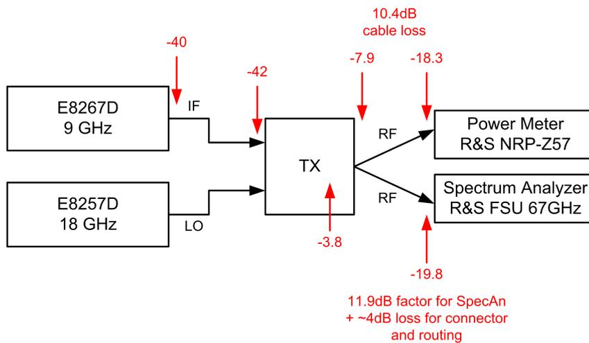
Figure 7.41: Test and calibration setup for GTC3 measurements.
