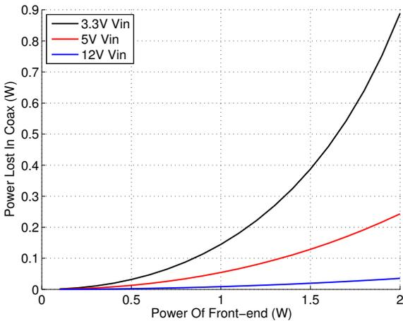
**Figure 7.24:** Power lost over the coax cable, assumes fixed 1ohm  $R_{tot}$
