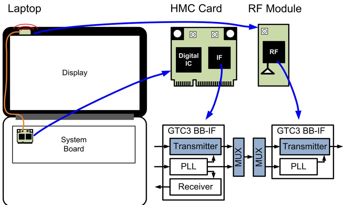
**Figure 7.2:** A two chip implementation for 60 GHz and placement in laptops.
