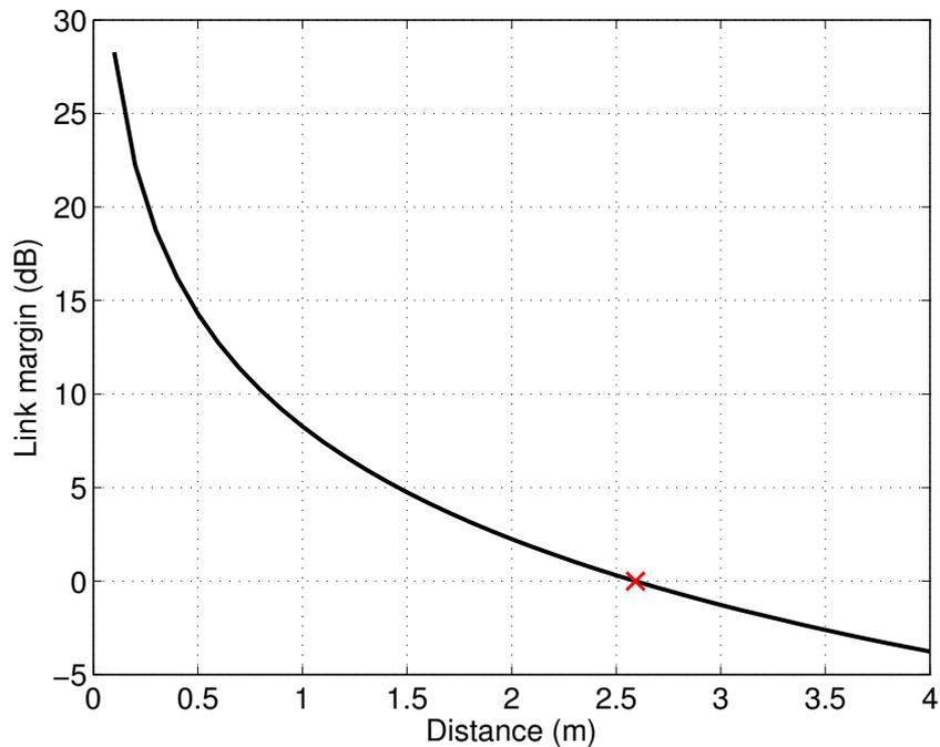
**Figure 7.4:** AWGN link margin in dB versus distance for 1x1 QPSK 2Gbps link. TX EIRP 12dBm, antenna gain 3dBi each side, RX NF of 10dB, SNR requirement of 10dB.
