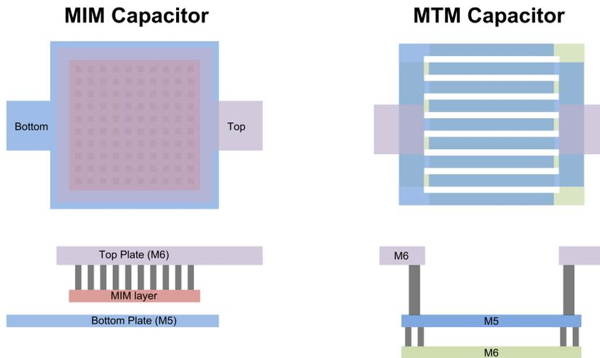
**Figure 2.4:** *MIM and MTM capacitors in a Silicon technology.*
