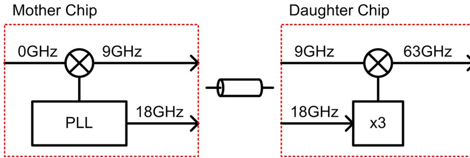
Figure 7.26: Frequency Plan for Split-IF Architecture
