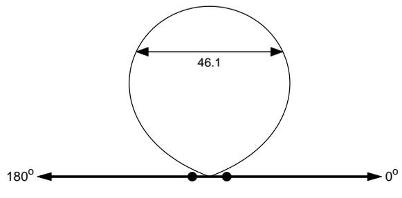
Figure 3.21: 2 element linear array factor,  $\frac{\lambda}{2}$  spacing
