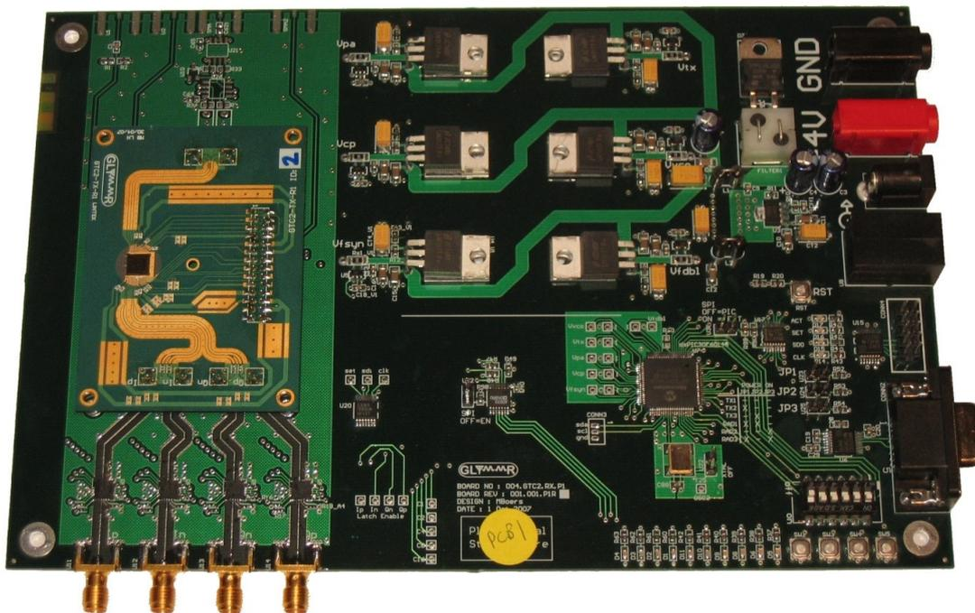
**Figure 7.13:** Development boards designed for testing the transmitter
