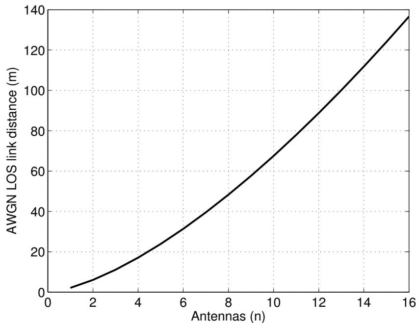
Figure 7.22: Link distance versus number of antennas for a QPSK LOS 60 GHz link.
