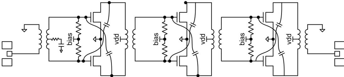
Figure 6.10: Block diagram of the transformer-coupled CMOS PA.
