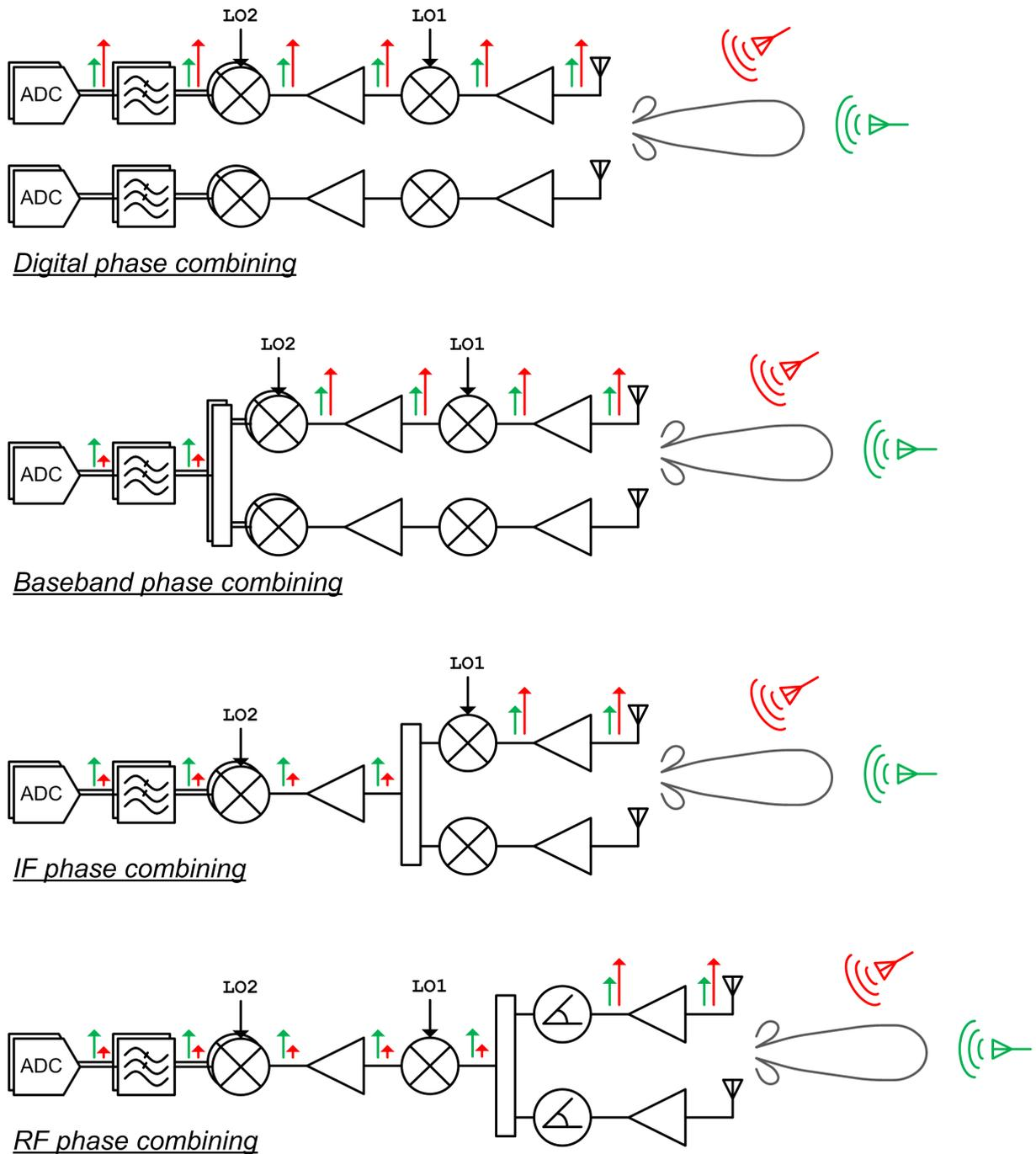
Figure 3.26: Phased Array Architectures
