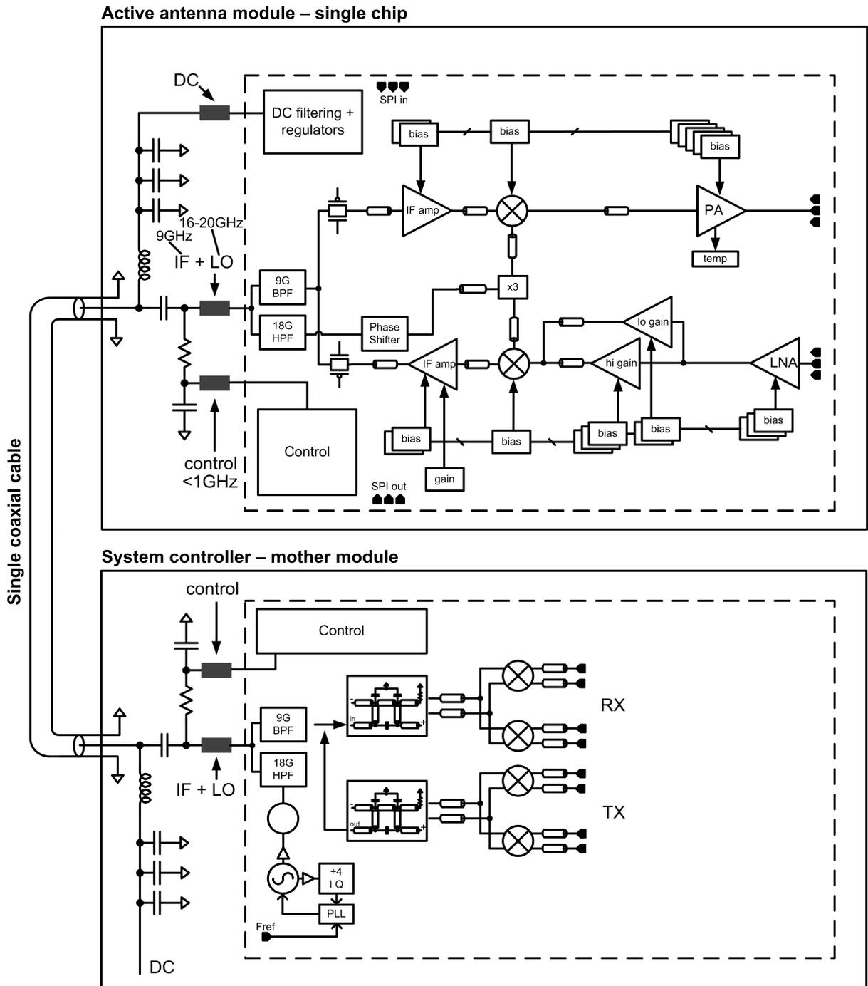
**Figure 7.27:** High level block diagram for GTC3 system. The transmitter is covered in this chapter. The receiver was designed by Leonard Hall and James Howarth. The PLL was designed by Yingbo Zhu and Noorfazila Kamal.
