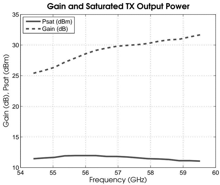
Figure 7.16: Gain and Saturated Output Power for GTC2-Tx.
