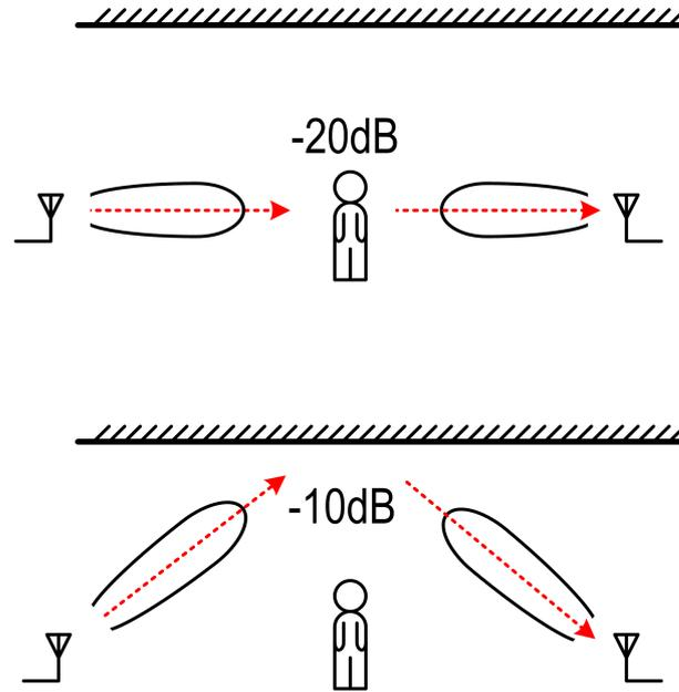
**Figure 4.2:** A blocked LOS link is shown at the top. In this link, the blocker has 20dB loss. In a beam-formed system, it is better to steer around the blocker and use a reflected path. The loss due to reflection varies based on the material but 10dB has been found to be a reasonable approximation [16].
