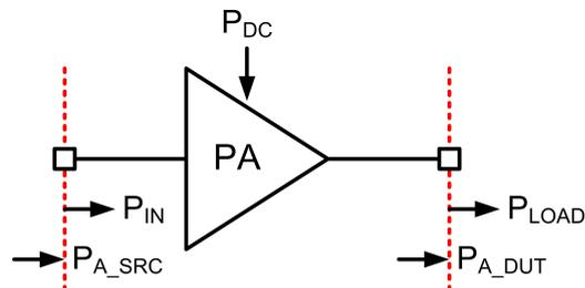
**Figure 5.2:** PA with annotated power definitions.
