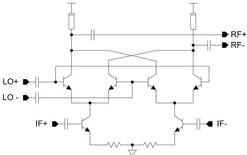
Figure 7.9: Block diagram of SiGe RF mixer
