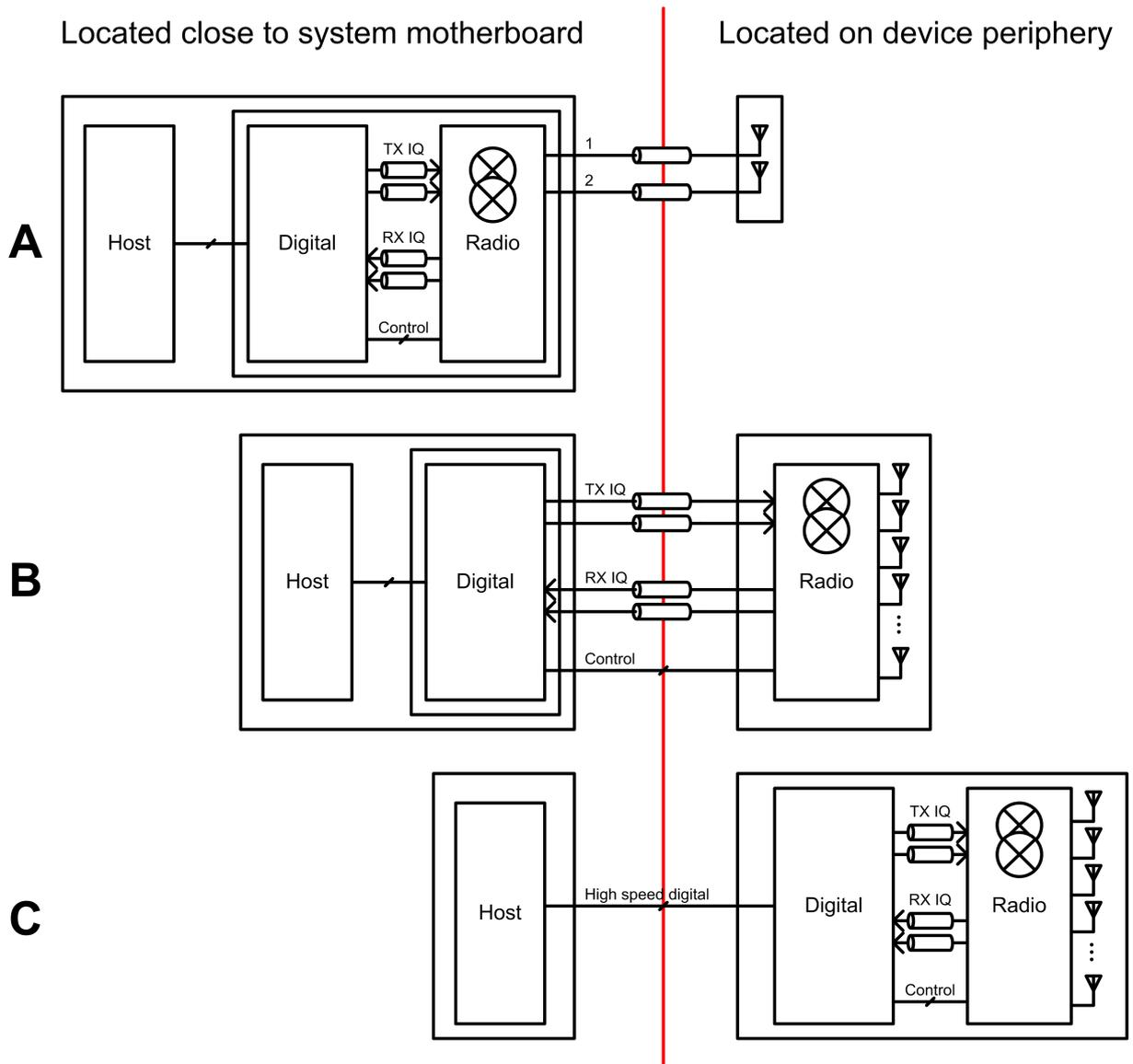
Figure 7.20: Typical architectures for wireless communication systems
