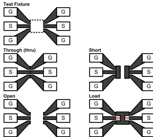
**Figure 5.9:** Test fixture and SOLT structures for chip level design.
