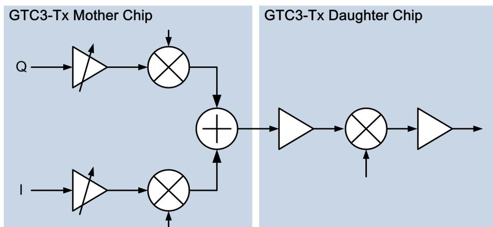
Figure 7.28: Block diagram of the GTC3 transmitter.
