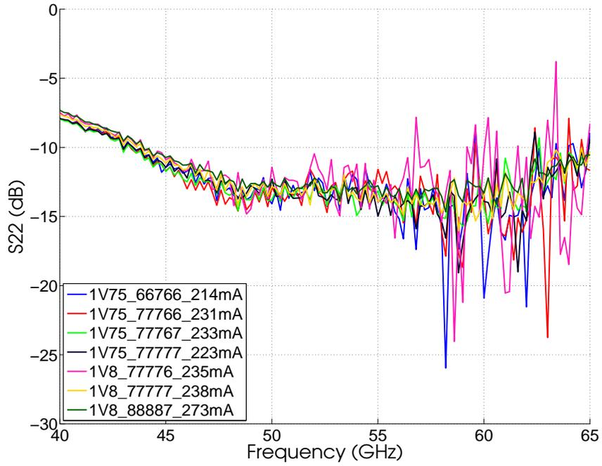
Figure 5.28: GTC2 PA S22 plot.
