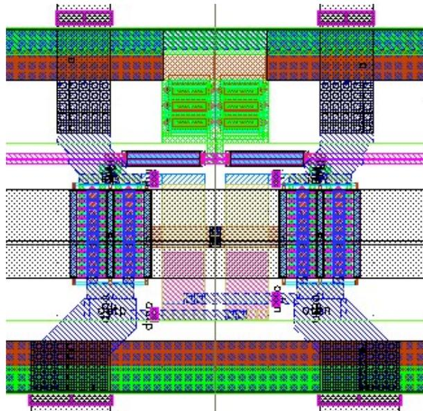
**Figure 6.14:** Transistor layout showing neutralisation capacitors.
