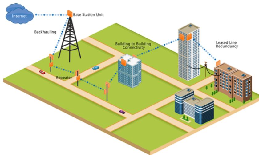
Figure 1.4: 60 GHz for wireless backhaul [12].
