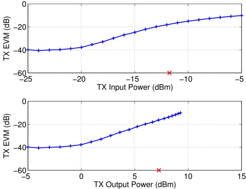
**Figure 3.16:** Plots showing TX EVM versus input and output power. An EVM floor of  $-40\text{dB}$  is assumed.
