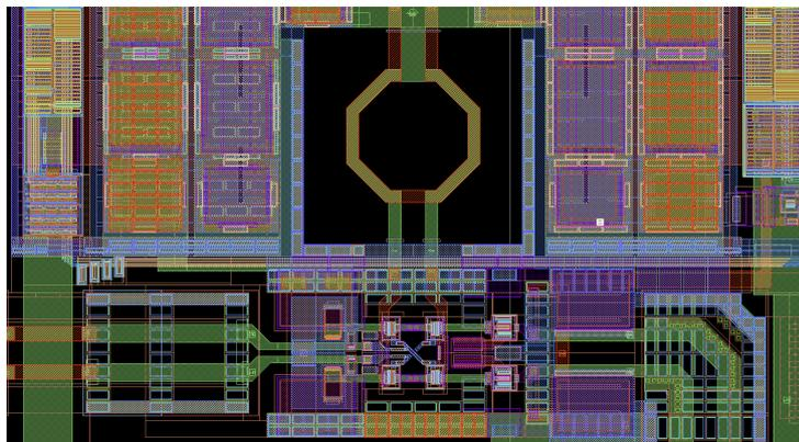
Figure 7.34: Layout of IF to RF mixer
