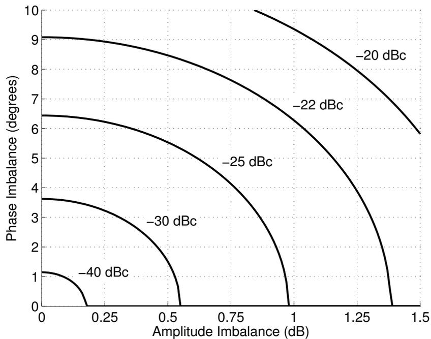
**Figure 3.9:** Amplitude (dB) and phase (degree) imbalance curves for different sideband suppression (dBc) levels.
