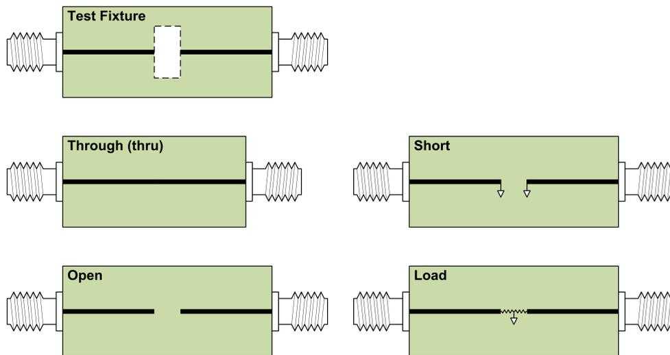
**Figure 5.8:** Test fixture and SOLT structures for board level design.
