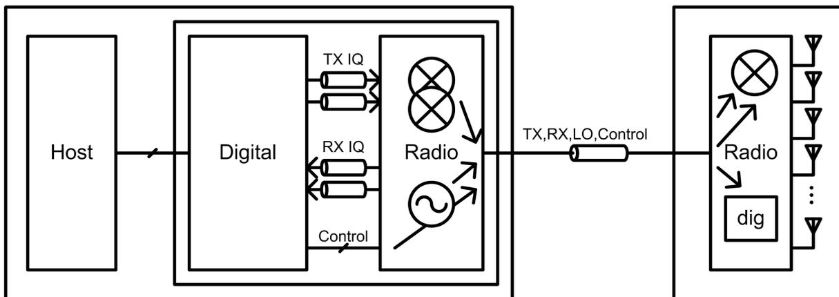
**Figure 7.21:** Proposed Split-IF Architecture - Taped out in January 2009.
