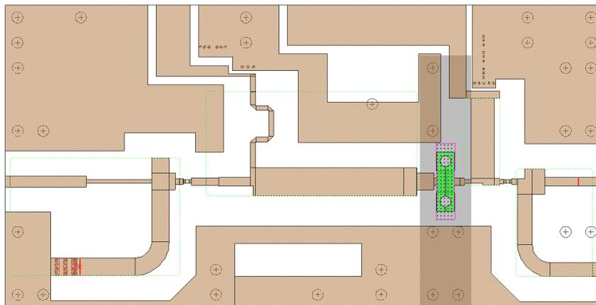
**Figure 5.16:** Final layout for the amplifier.
