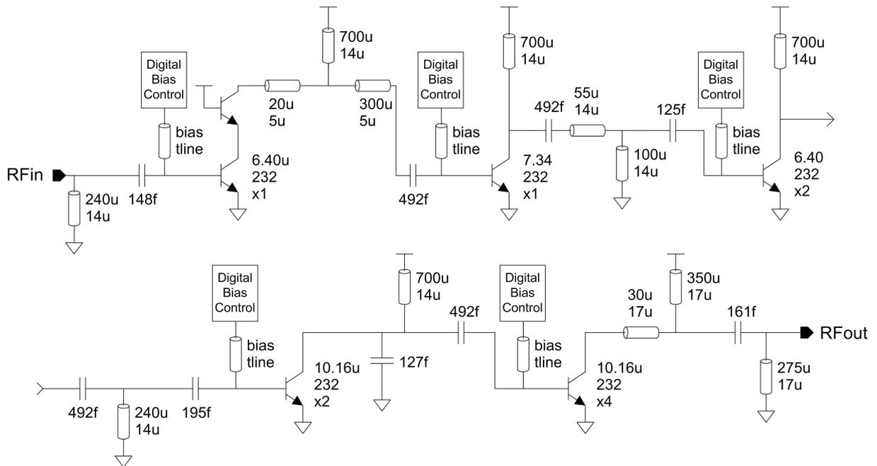
Figure 5.22: Block diagram of the SiGe PA.
