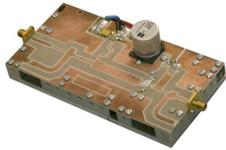
1 GHz high efficiency GAN HEMT board level PA. The PA uses a GAN HEMT device. The boards were manufactured by Macquarie Engineering and Technical Service.
