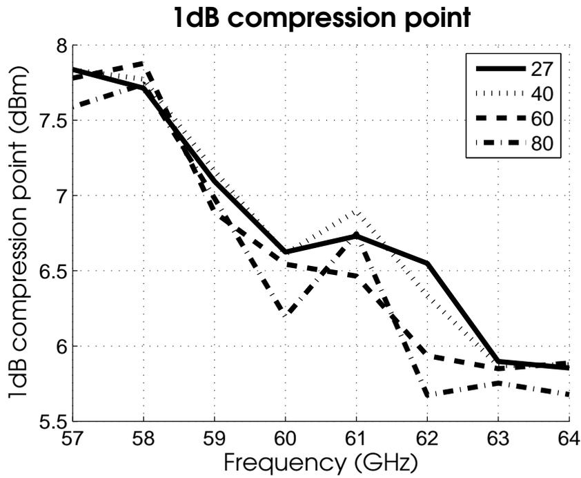
Figure 6.18: Output 1dB compression point.
