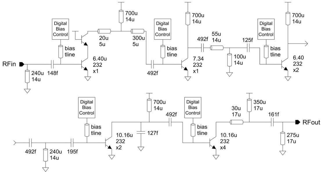
**Figure 7.6:** Block diagram of 0.18  $\mu\text{m}$  Jazz SiGe transmission line PA used in GTC2-Tx.
