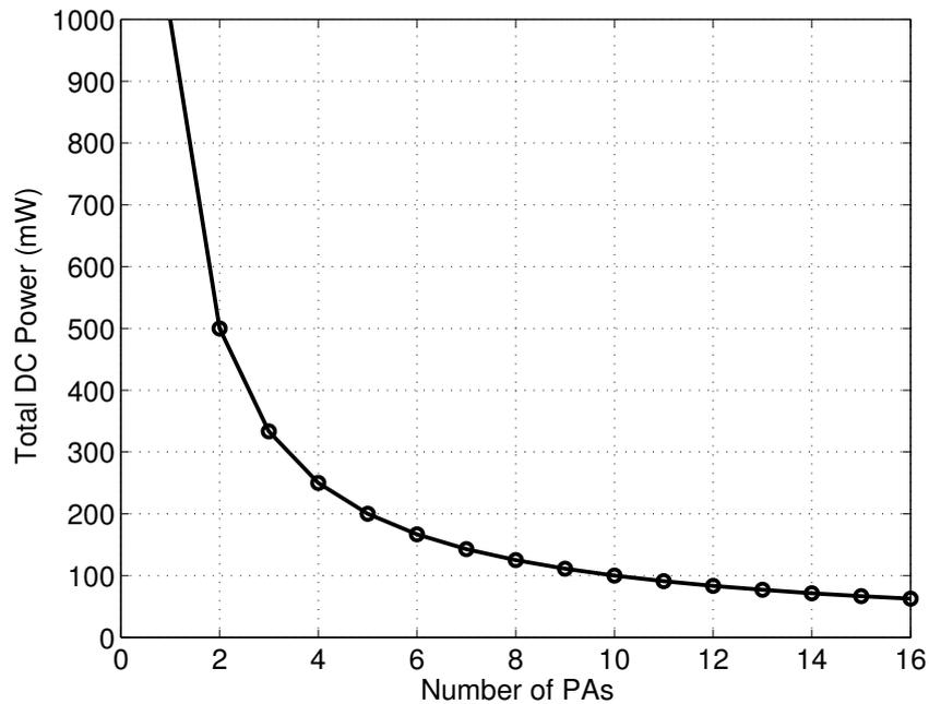
**Figure 5.6:** Total power to achieve a 20dBm EIRP assuming 10% PA efficiency.
