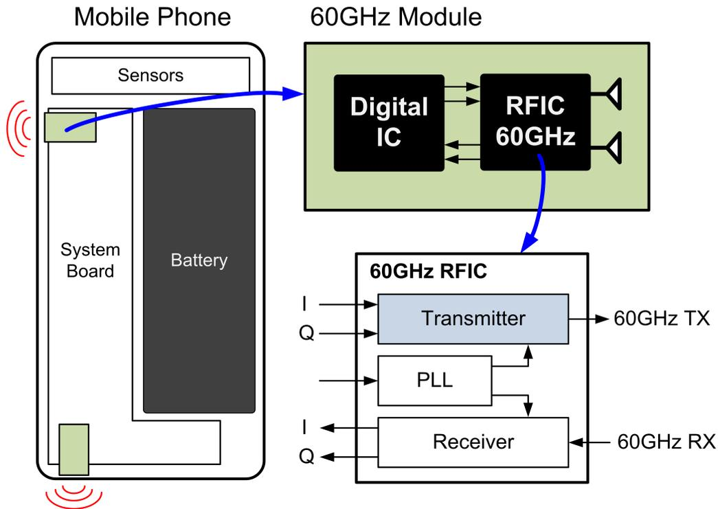
**Figure 7.1:** A single chip implementation for 60 GHz and placement in mobile phones.
