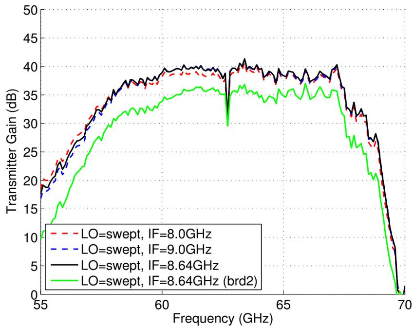
**Figure 7.49:** *Transmitter gain with swept LO signal, this shows the frequency response of the RF front-end. A second chip is measured which shows the same response, just slightly lower output power likely due to variation in the wire-bonding.*
