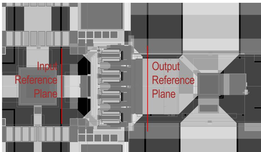
**Figure 5.24:** *Layout of the output stage transistors.*
