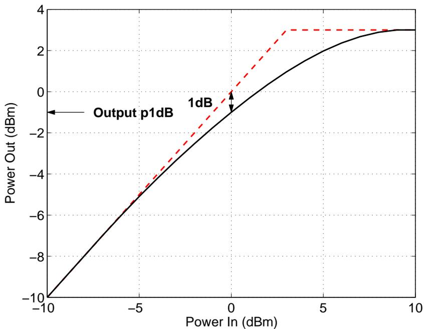
**Figure 3.13:** *Output 1dB compression point definition.*
