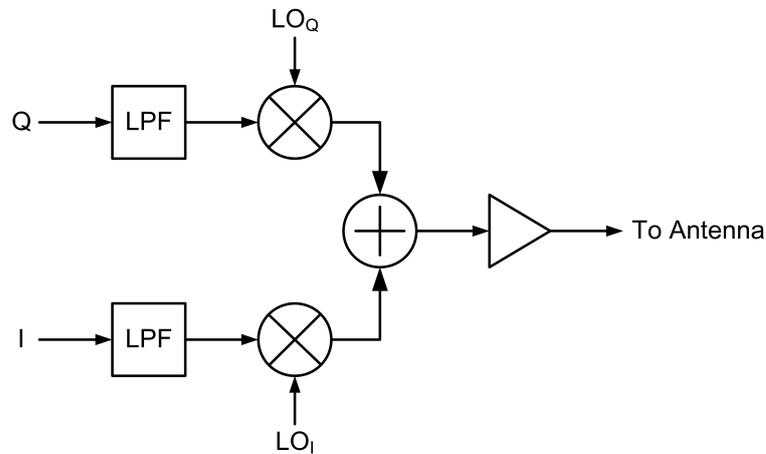
**Figure 3.2:** *Direct-conversion transmitter.*
