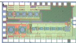
0.18 μm SiGe modular 60 GHz front-end transmitter for split IF single coaxial cable system - GTC3-TX.
