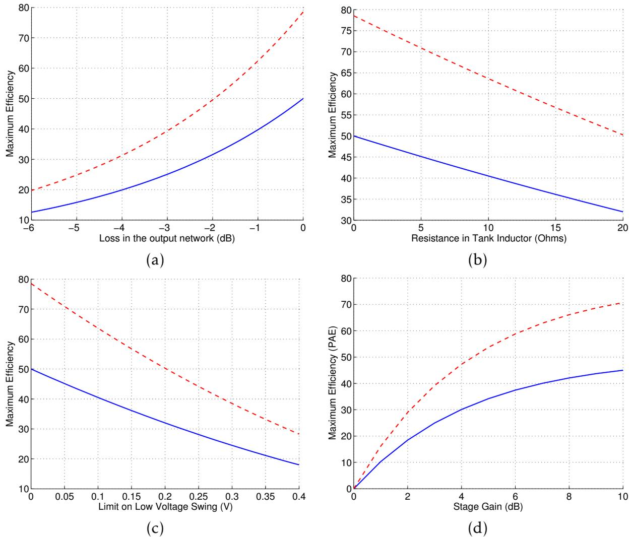
**Figure 5.5:** This set of plots show the maximum efficiency of a Class A (blue) and Class B (red dots) with ideal implementation except for (a) loss in the output network (b) resistance in the tank Inductor (c) limit on the available swing (due to knee or reliability limits) (d) the gain of the stage (in this case PAE is plotted)
