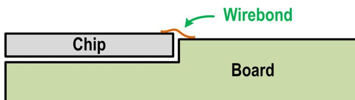
**Figure 7.14:** *The chip is inserted into a cavity on the PCB to reduce the length of the wirebond.*
