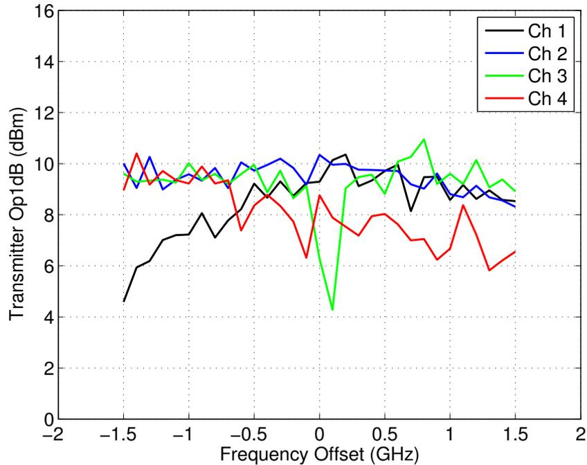
**Figure 7.45:** Relative TX output 1dB compression point for each 802.11ad channel.
