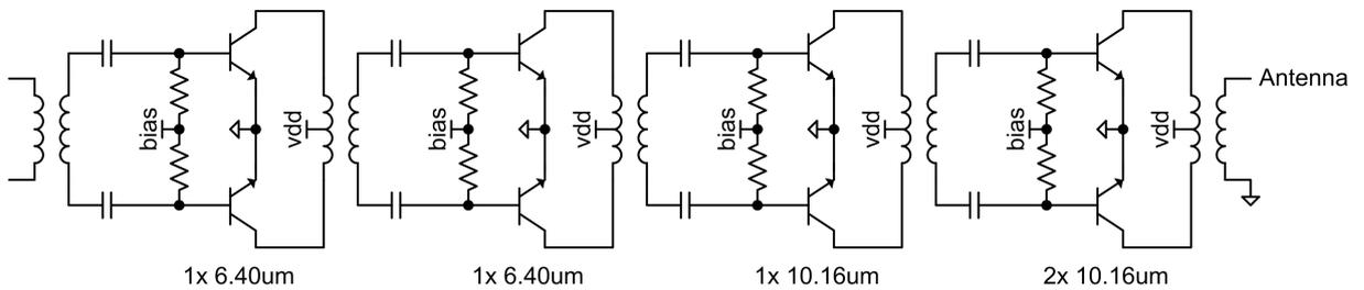
**Figure 6.2:** Schematic of PA
