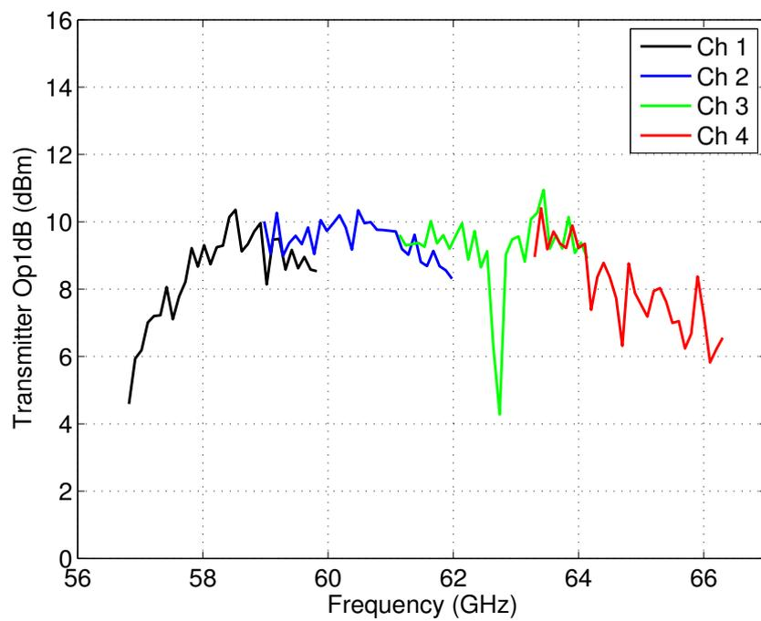
Figure 7.44: TX output 1dB compression point for each 802.11ad channel.
