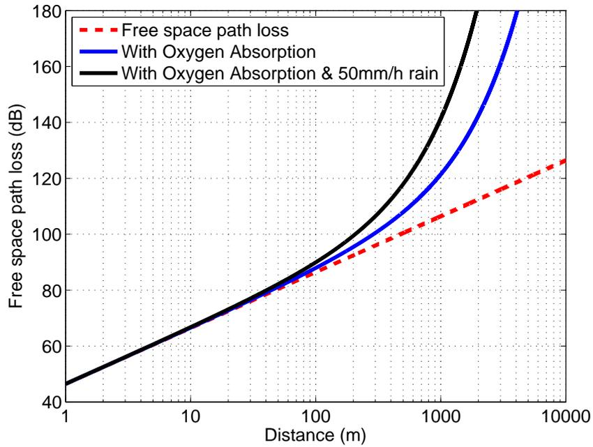
**Figure 1.6:** Free space path loss at 60 GHz. The loss including Oxygen absorption and rain is also shown (Rain fall data from [14]).
