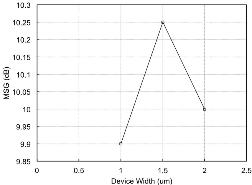
Figure 5.11: Transistor MSG (dB) vs. device finger width (um). Total device size is constant (90um).
