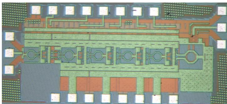
**Figure 6.7:** Standalone PA for testing. Approx 1.1mm x 0.5mm.
