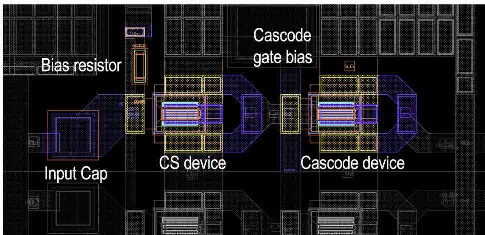
Figure 6.4: GTC3 PA input cascode stage.
