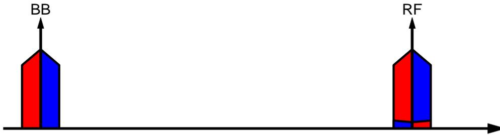
**Figure 3.3:** Up-conversion in a direct conversion transmitter. The complex (I/Q) signal at baseband (BB) is up-converted directly to RF using an LO at the centre of the RF channel.
