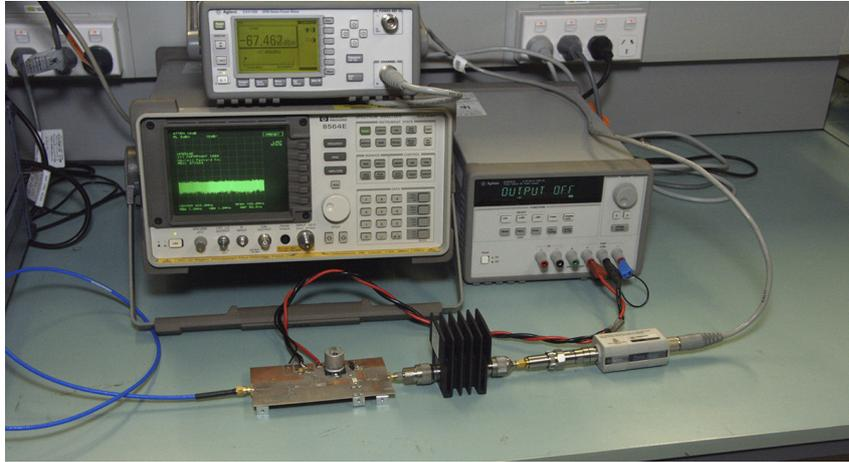
**Figure 5.20:** Testing a prototype at Macquarie University (photo courtesy of Professor Anthony Parker). The board is implemented using a Rogers substrate.
