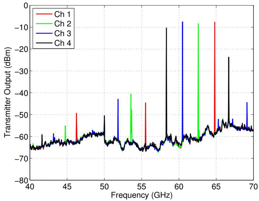
**Figure 7.46:** Output spectrum for each channel showing lower image, LO signal and upper image.
