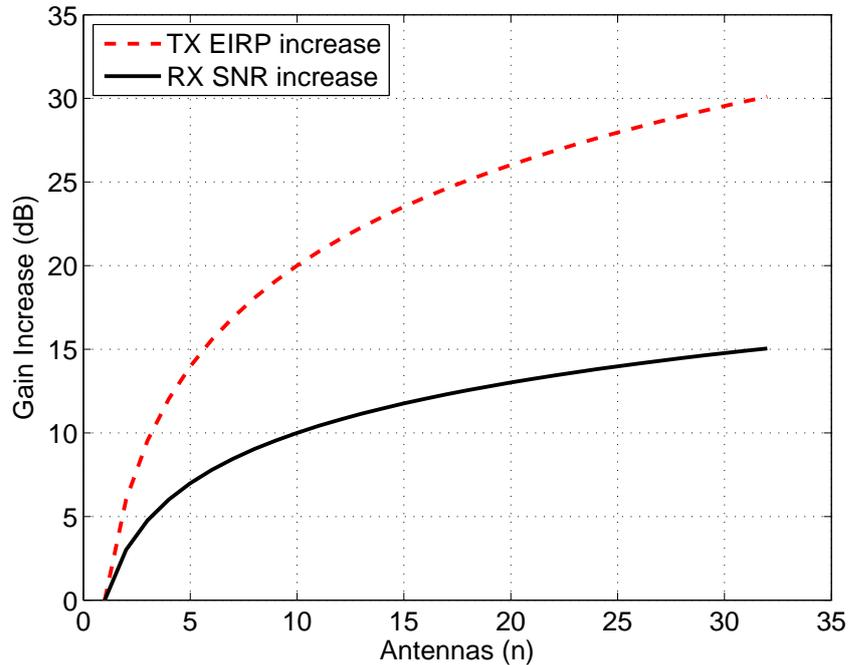
Figure 3.25: TX EIRP and RX SNR increase vs. Antennas
