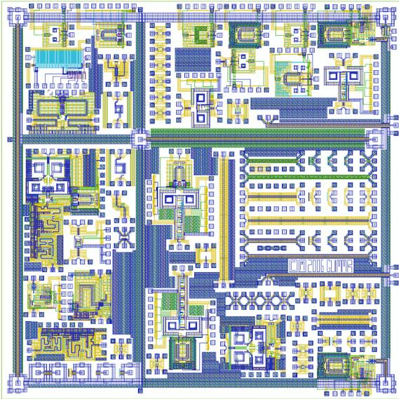
**Figure C.1:** *GLIMMR test-chip 1 (GTC1).*
