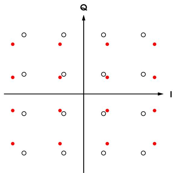
**Figure 3.8:** 16-QAM constellation with 3dB amplitude imbalance in I/Q paths.
