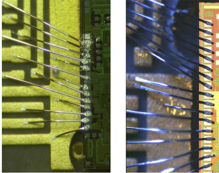
**Figure 7.15:** *On the left too much pressure was used for wirebonding, the right shows better bonds.*
