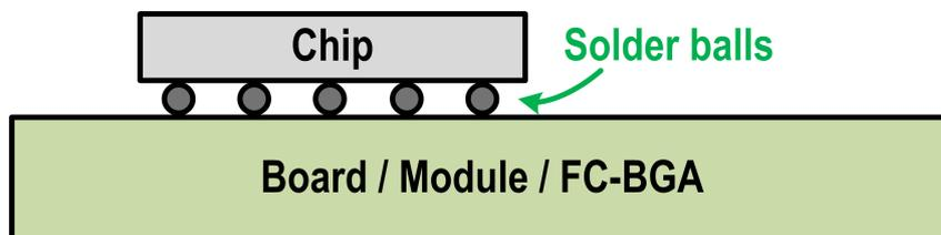
**Figure 2.9:** *Solder balls from chip to board, module or FC-BGA package.*
