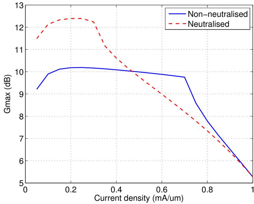
**Figure 6.13:** The  $G_{max}$  for both a neutralized transistor and a common-source configuration is shown. The  $G_{max}$  of the transistor with neutralization is 2.5dB higher than without.
