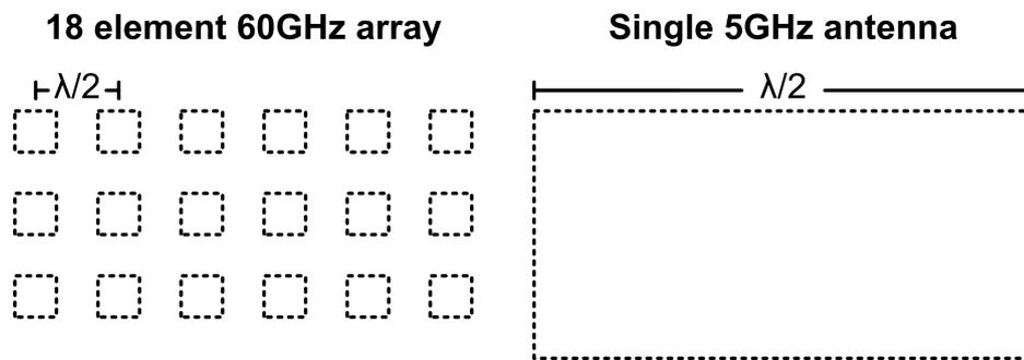
**Figure 3.1:** Simple comparison of size between 60 GHz and 5 GHz antennas
