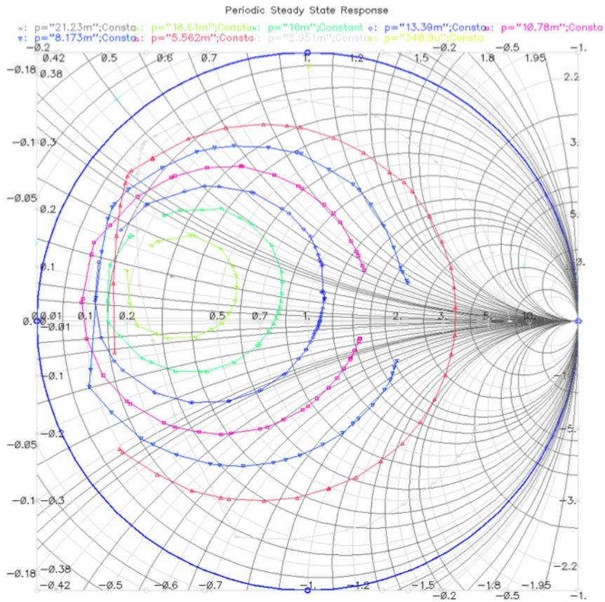
Figure 6.3: GTC3 output stage load pull simulation.
