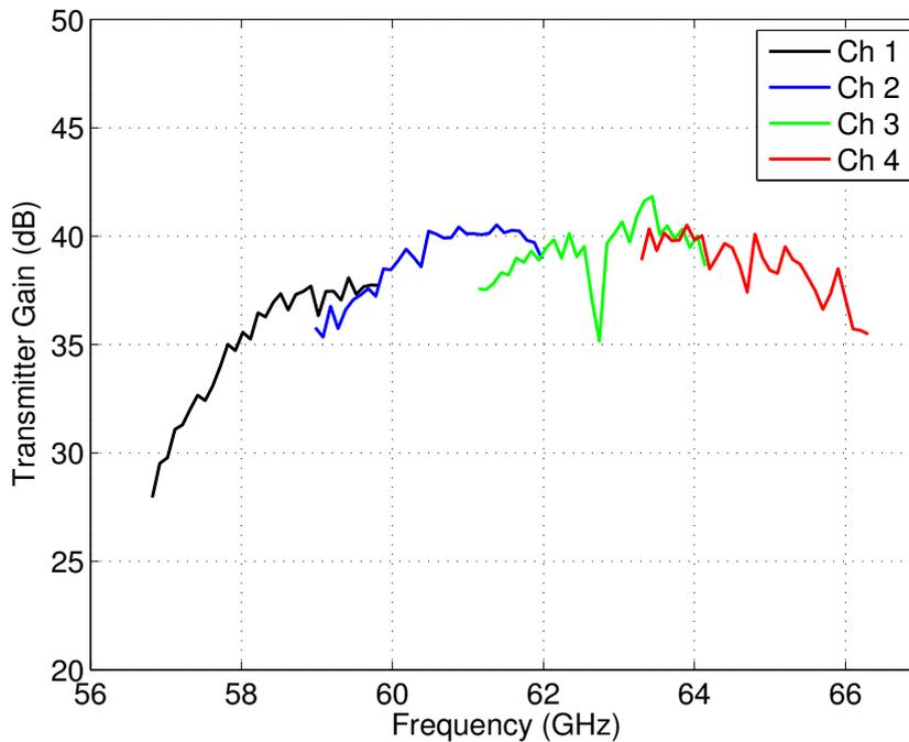
**Figure 7.42:** TX gain for each 802.11ad channel.
