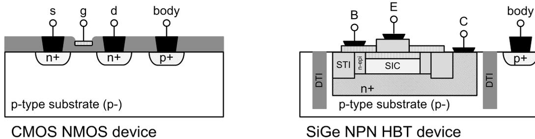
**Figure 2.2:** Cross section of NMOS (left) and NPN HBT (right) [34].
