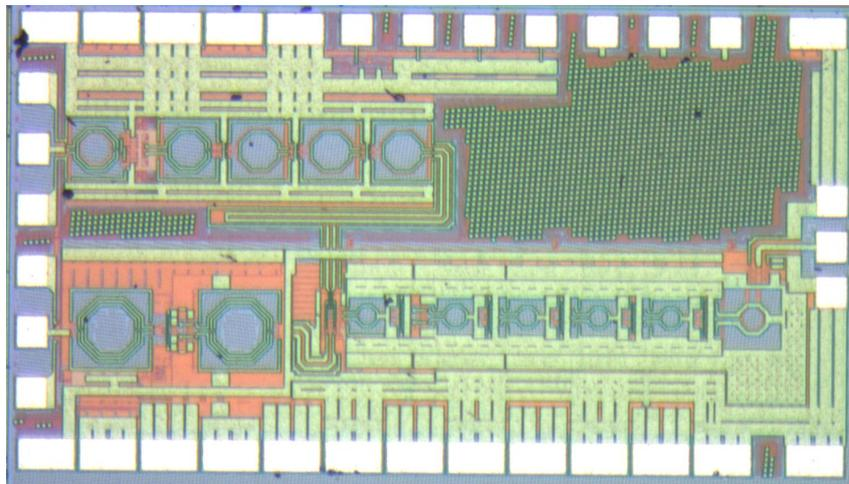
**Figure 7.37:** Chip micro-graph for IF to RF chip
