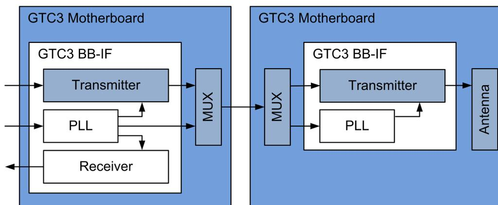
**Figure 7.19:** Simple diagram of GTC3 showing the areas covered in this section.
