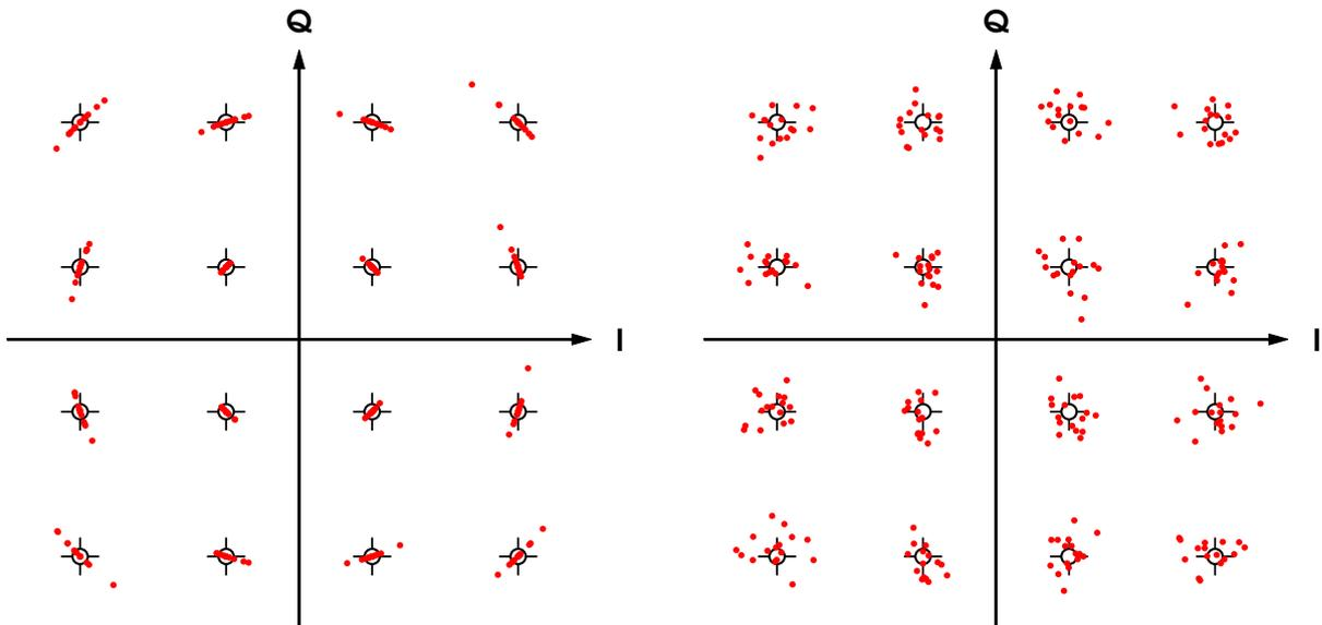
**Figure 3.11:** 16-QAM constellation with phase noise.
