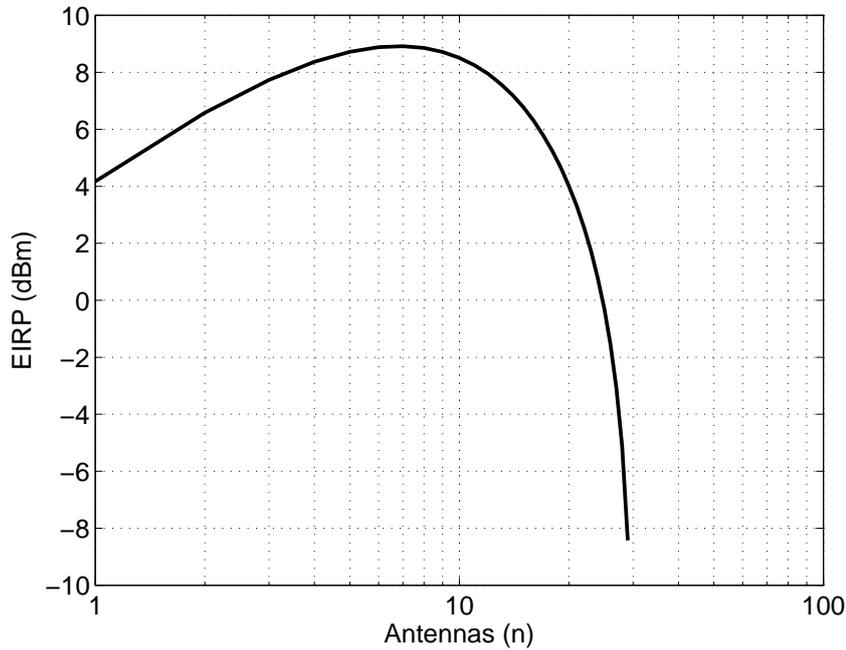
**Figure 4.4:** Total EIRP vs. number of TX antennas for a fixed power budget
