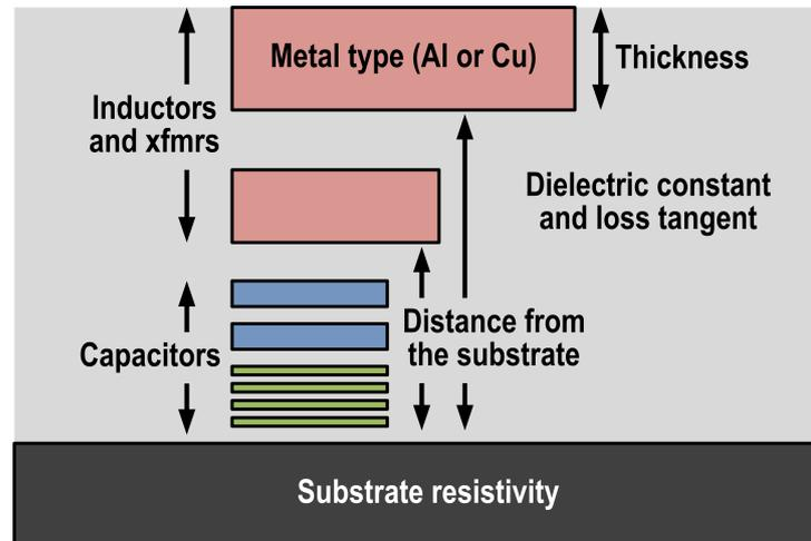
**Figure 2.7:** The left shows the metals used for different passive devices. The right highlights some of the main metal stack parameters which impact performance.
