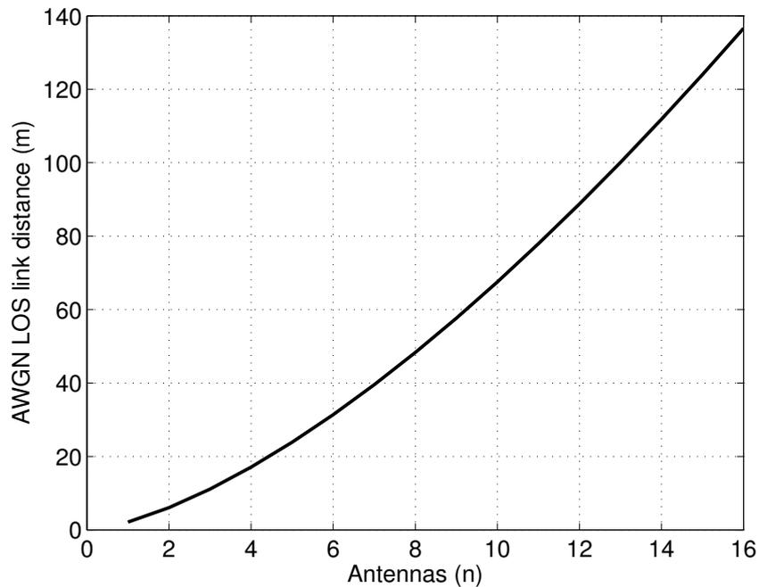
**Figure 4.1:** LOS link distance in an AWGN channel for increasing antennas
