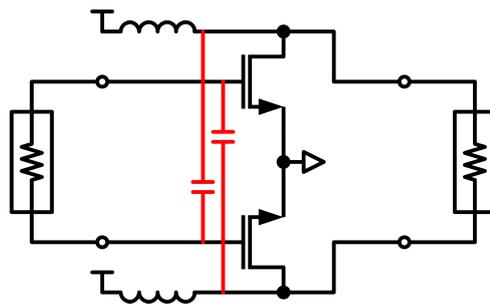
**Figure 6.12:** *Differential devices with neutralisation capacitors shown in red.*
