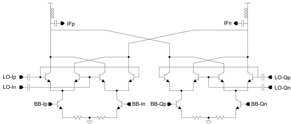
**Figure 7.7:** Block diagram of SiGe I/Q mixer used in GTC2-Tx.
