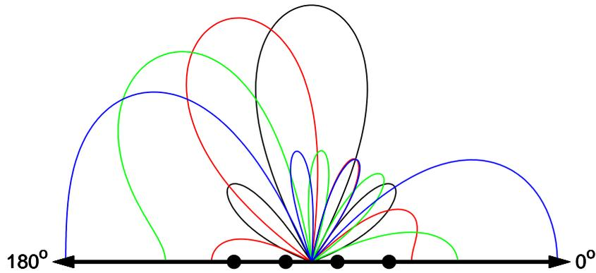
**Figure 3.24:** 4 element array,  $\frac{\lambda}{2}$  spacing, steering from 90 to 150
