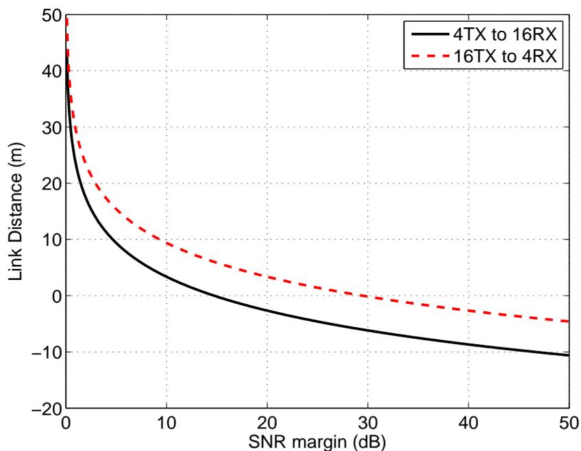
**Figure 4.5:** *Link SNR margin vs. distance for an asymmetric link setup*
