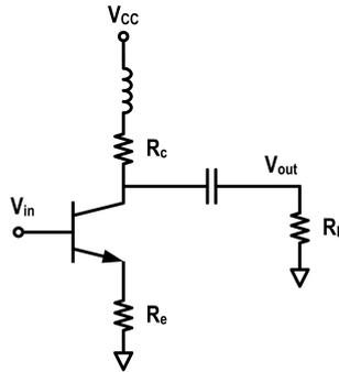
**Figure 5.4:** Example linear PA schematic.
