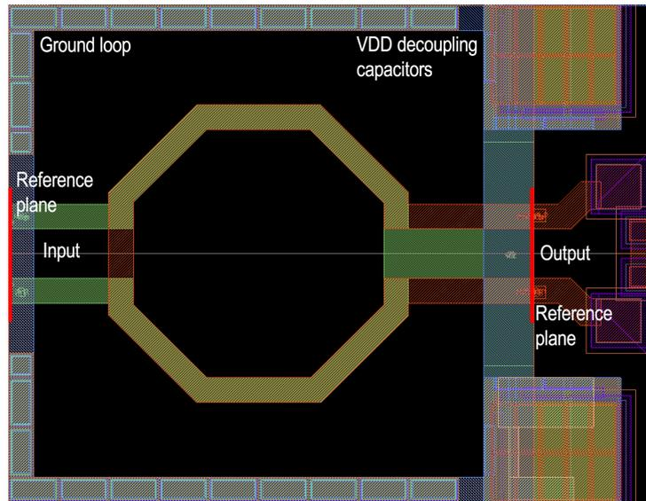
**Figure 6.5:** *Interstage transformer in GTC3 PA.*
