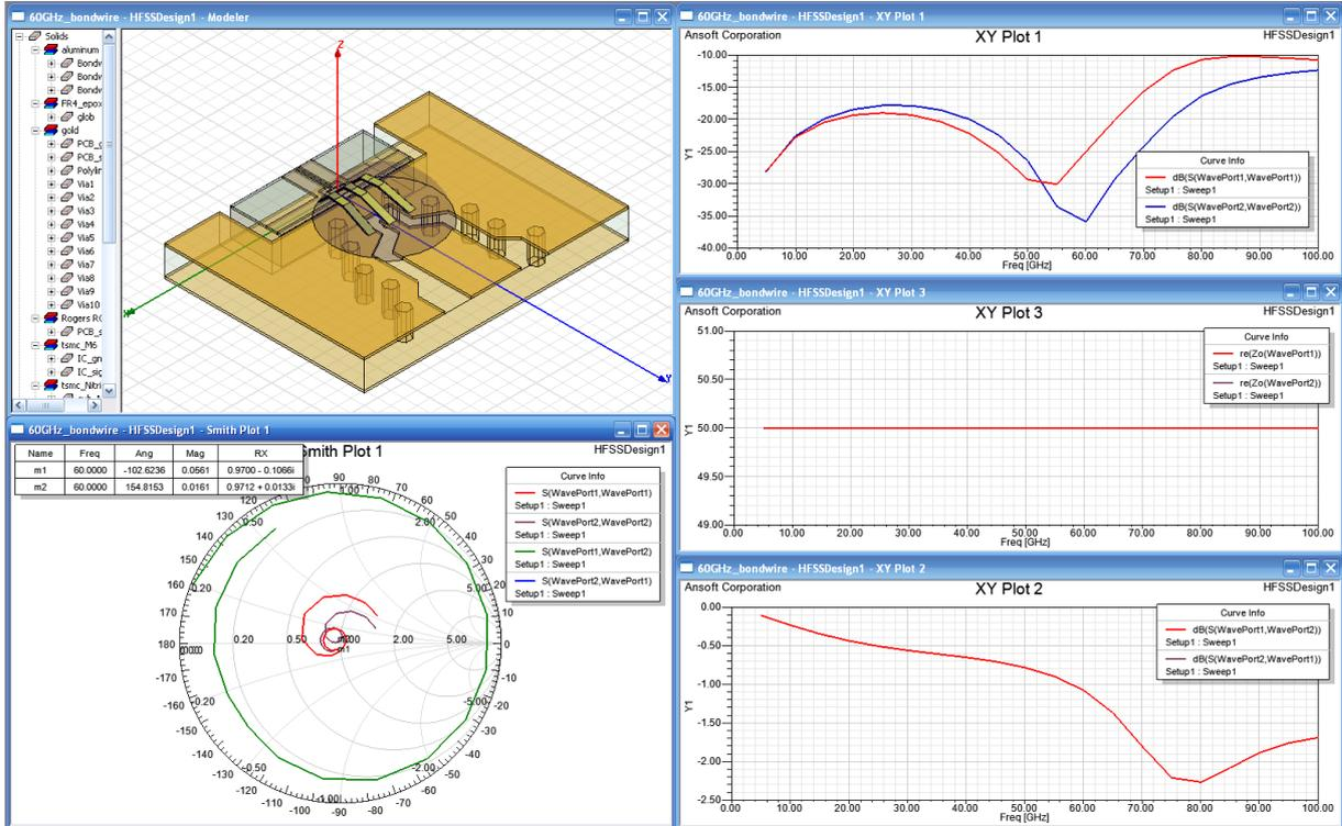
Figure 7.40: HFSS simulation of the wirebond for GTC3-Tx module
