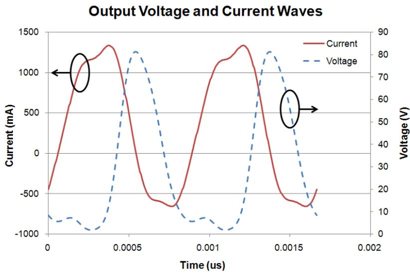
Figure 5.19: Output voltage and current waves.
