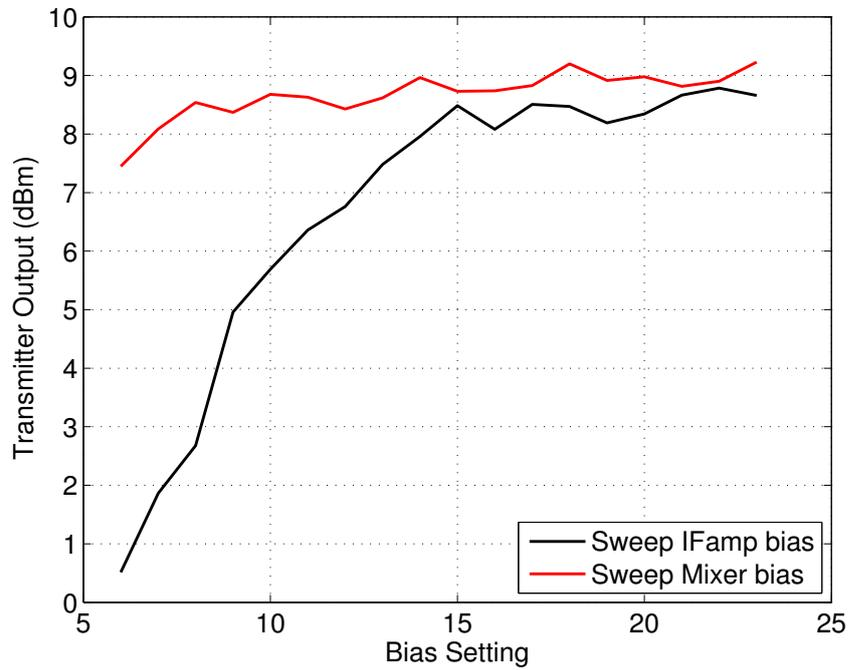
**Figure 7.48:** *Op1dB compression point versus IFamp and mixer bias settings.*
