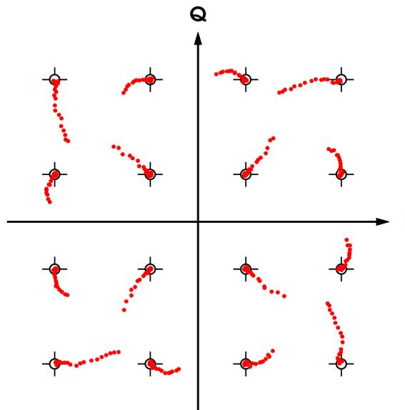
**Figure 3.15:** 16-QAM constellation pushed into hard compression. The PA is pushed to saturation. The power of each constellation is normalised.
