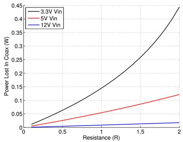
**Figure 7.25:** Power lost over the coax cable, assumes fixed 1W front-end power
