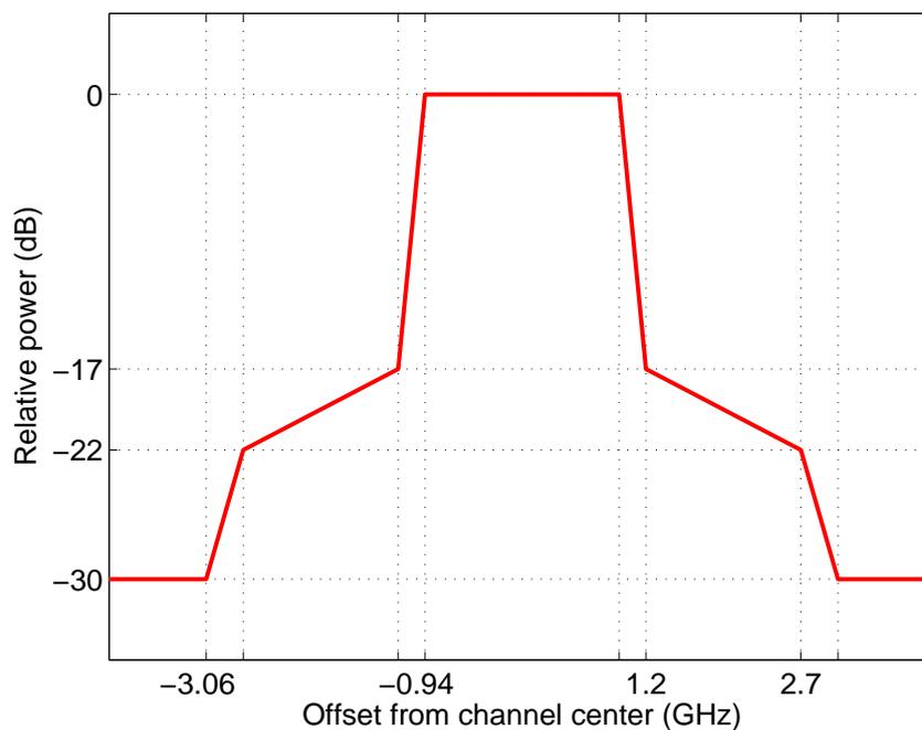
**Figure 3.17:** 802.11ad spectral mask [9].
