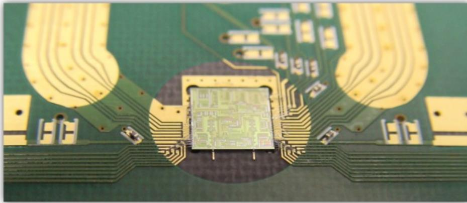
**Figure 7.12:** RF daughter board for TX testing. Board designed by the author, antennas by Leonard Hall.
