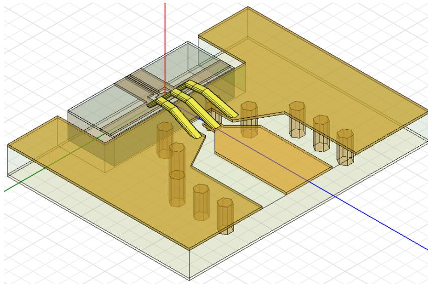
**Figure 2.8:** *High frequency bond-wire transition.*
