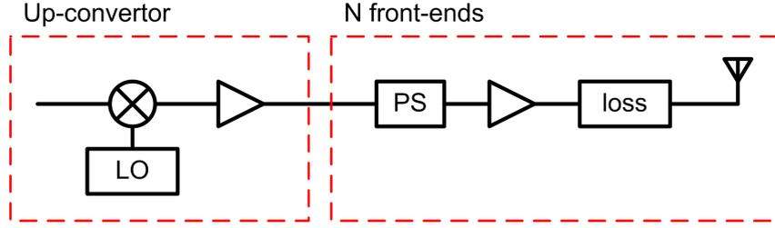
Figure 4.3: Simple transmitter block diagram
