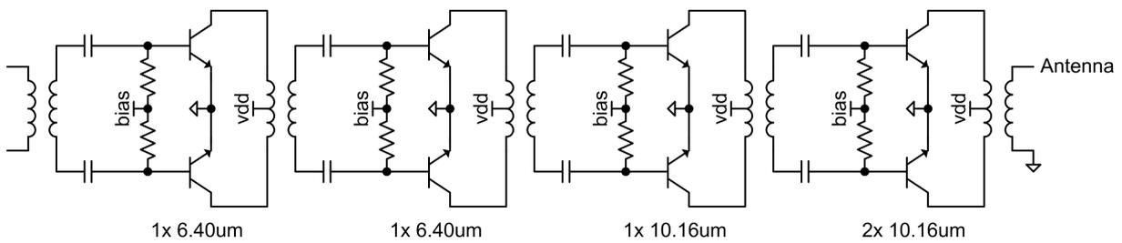
Figure 7.35: Schematic of Power Amplifier
