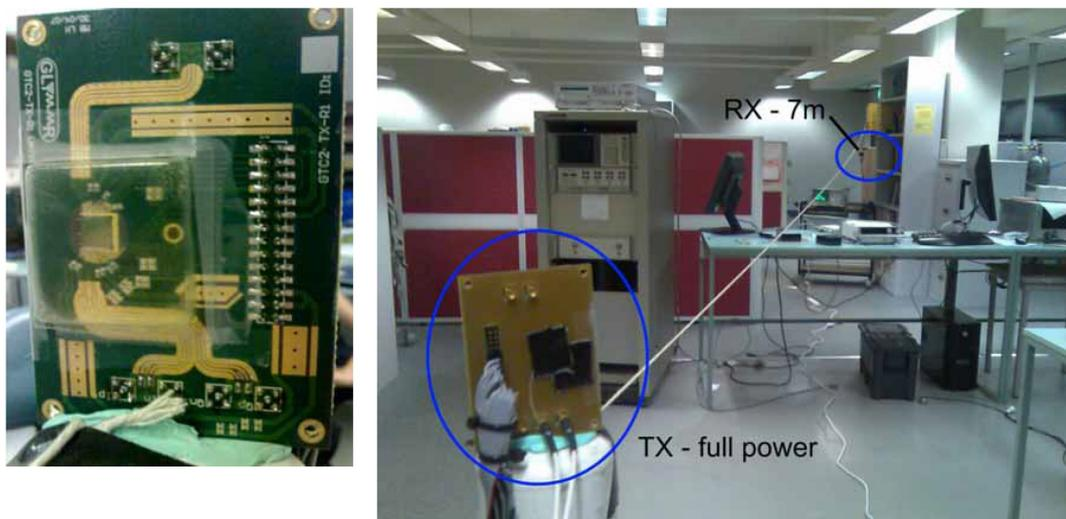
**Figure 7.18:** Photo showing TX to Spectrum Analyzer link experiment
