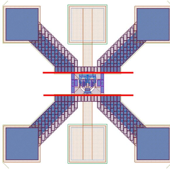
**Figure 5.13:** Transistor shown in test structure with reference plane defined in red.
