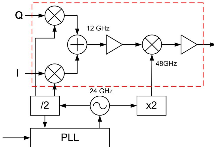
Figure 7.5: GTC2 block diagram.
