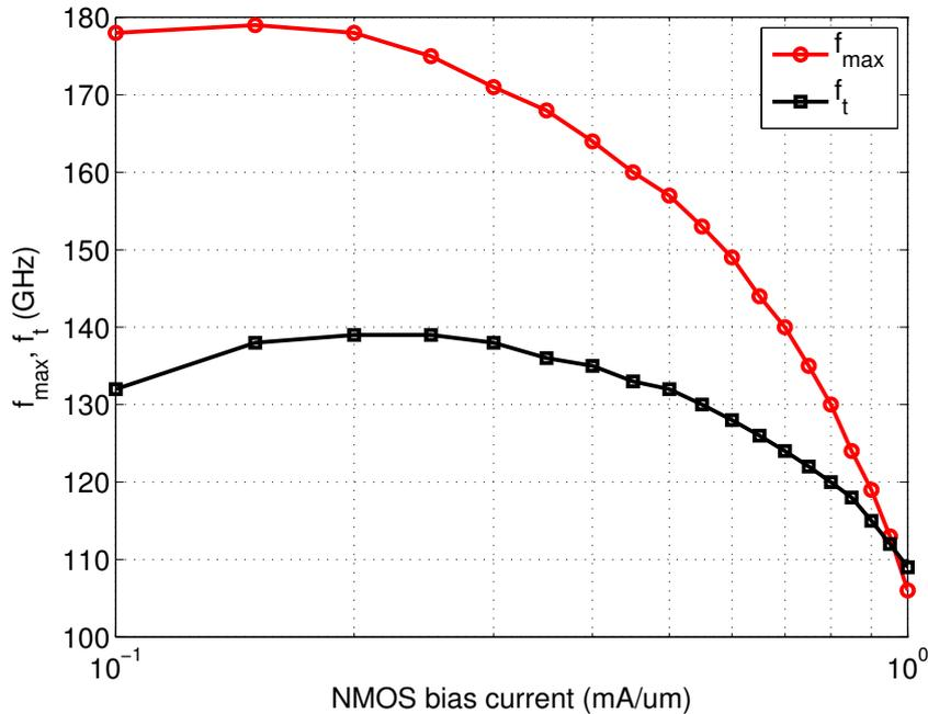
**Figure 5.12:** CMOS device  $f_T$  and  $f_{max}$  versus bias current.
