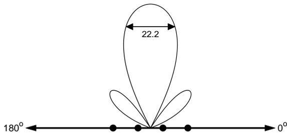
**Figure 3.22:** 4 element linear array factor,  $\frac{\lambda}{2}$  spacing
