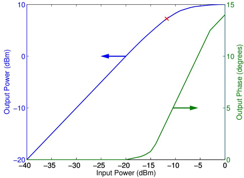
**Figure 3.14:** Example plot of *am-am* and *am-pm* characteristics for a transmitter.
