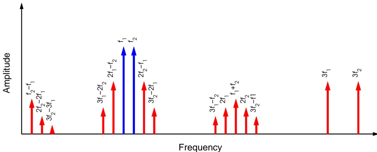
**Figure 3.18:** Two input frequencies  $f_1$  and  $f_2$  inter-modulate to create many output components.
