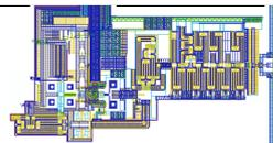
60 GHz 0.18 μm SiGe 1 element transmitter - GTC2-TX.
