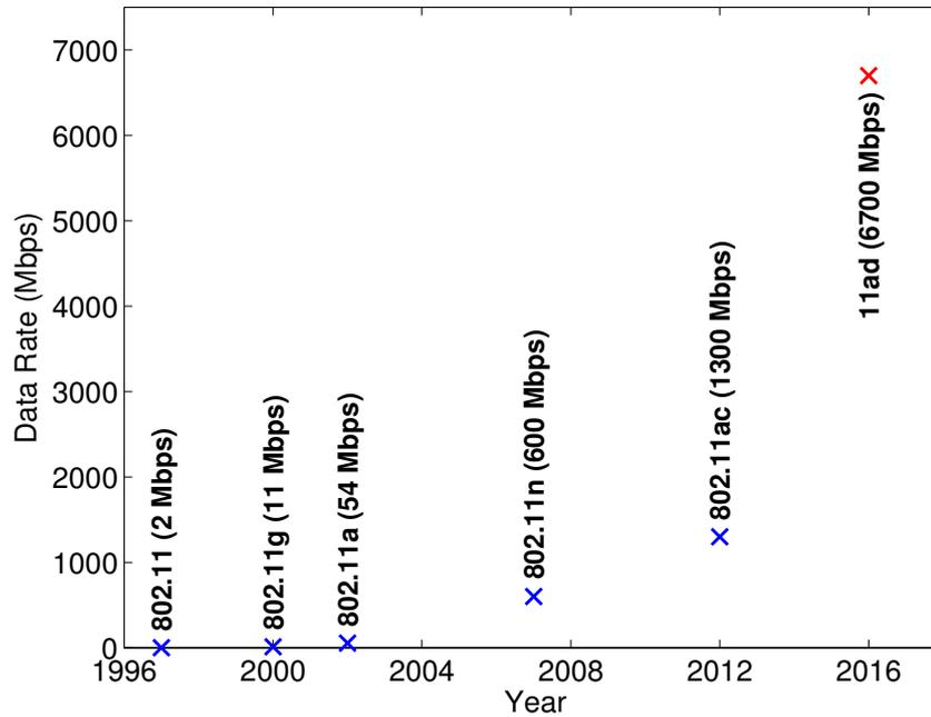
**Figure 1.1:** The 802.11 wireless evolution 11g to 11ad. The y-axis shows the highest PHY rate specified in the standard.
