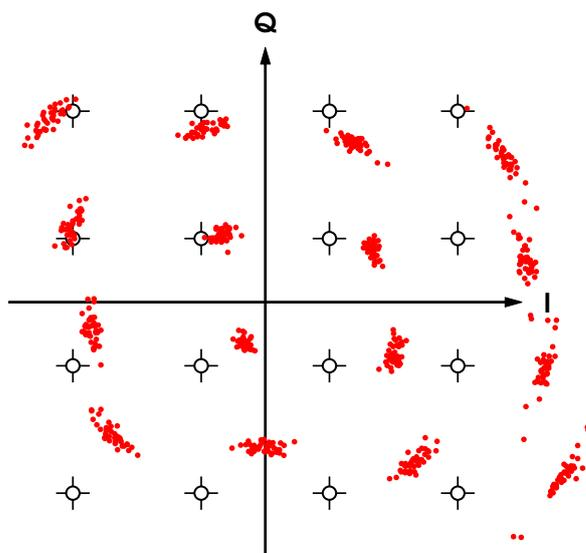
**Figure 3.19:** TX output constellation showing a combination of TX impairments.
