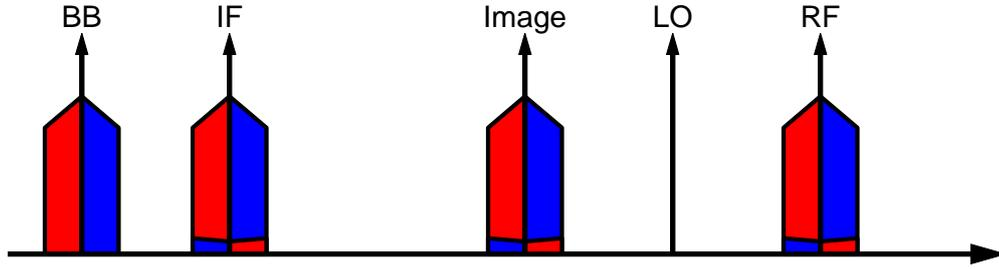
**Figure 3.5:** Up-conversion in a dual conversion transmitter. The complex (I/Q) signal at baseband (BB) is first up-converted to an IF and then converted to RF using an offset LO.
