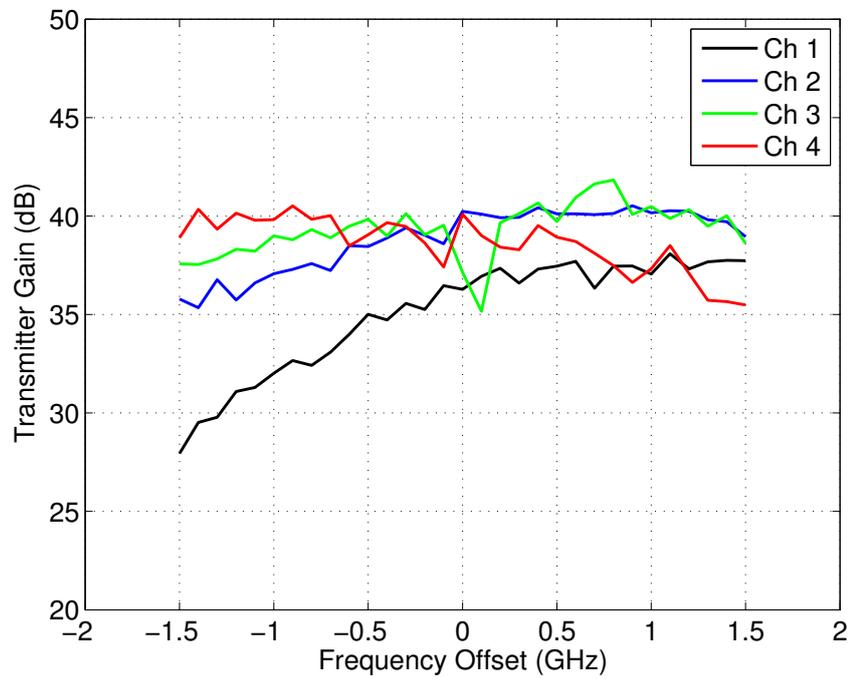
Figure 7.43: Relative TX gains for each 802.11ad channel.
