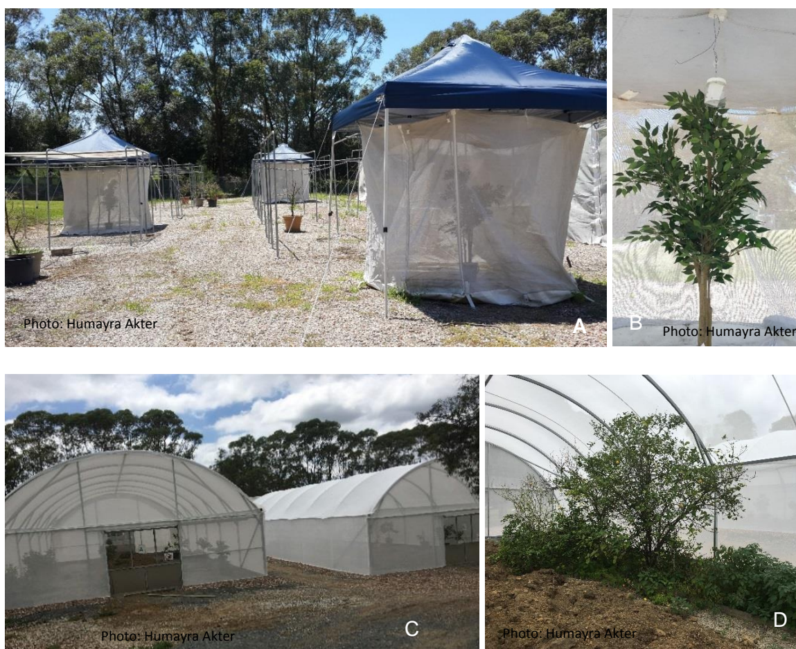
Figure 1. Field cages where experiments were run; (A-B) small field cage (3 m diameter, 2.2 m high) with 1 artificial plant and 1 lure trap and (C-D) large field cage (8 x 24 m) where citrus plants and both lure and control traps were suspended.
