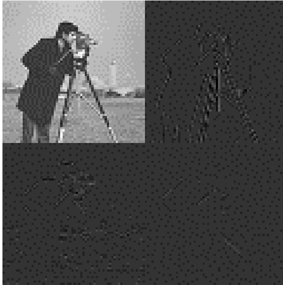
FIGURE 6.21: Camera-man image after one level of 2D processing using proposed image processor
