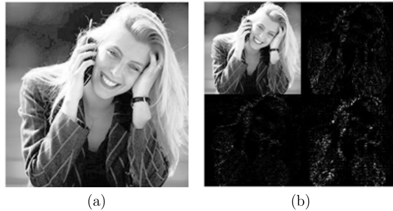
FIGURE 2.5: Lifting-based image compression: (a) Original image "phone.jpg" 256 \times 256 , (b) One level of lifting decomposition
