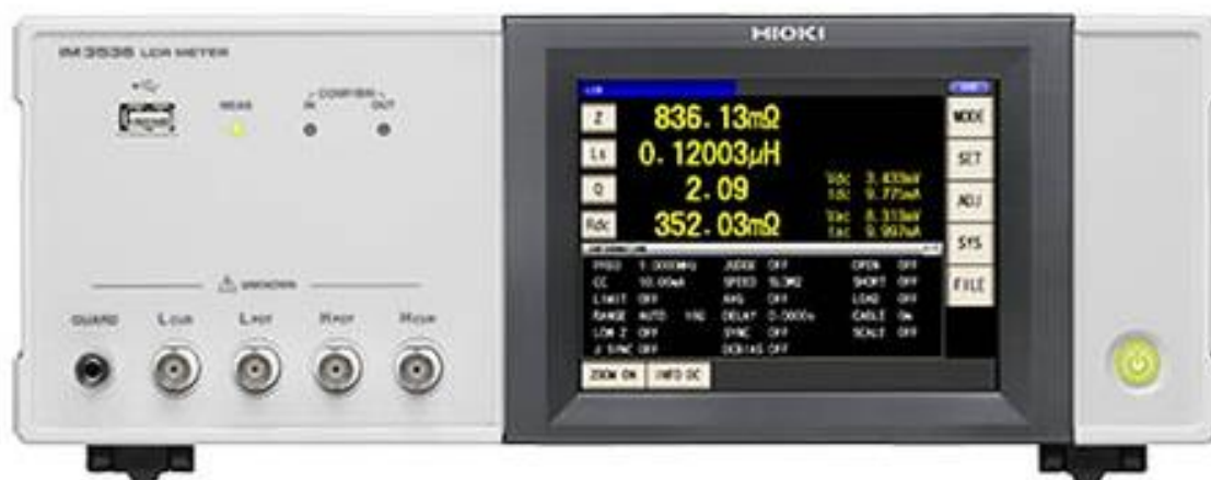
Figure 3.12 The front panel of a high precision HIOKI IM3536 LCR Meter (Japan) [153].
