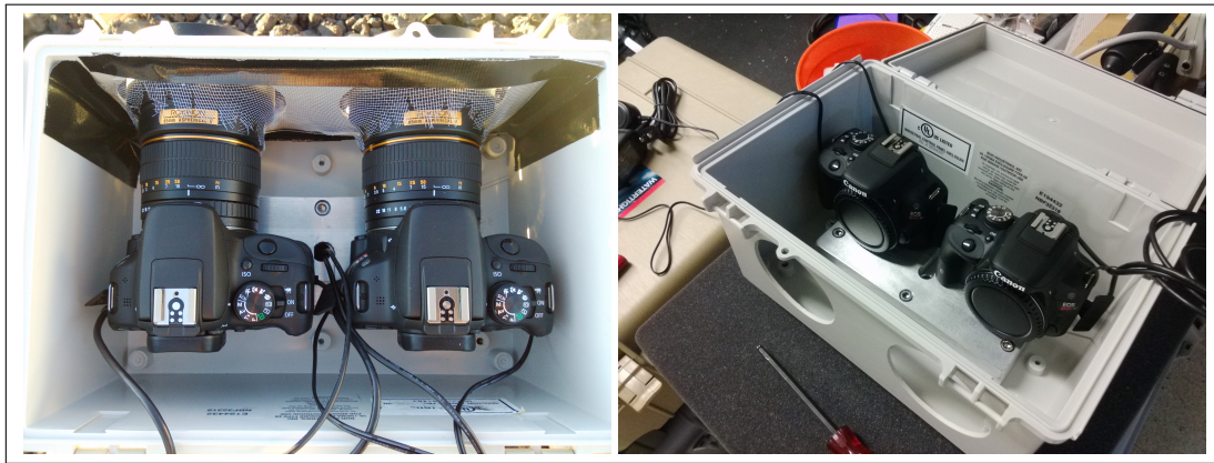
Figure 1.2: Left: Two Canon EOS 100D (Rebel SL1) with Rokinon 85mm f/1.4 lenses installed inside the PAN001 camera box. Right: Two of the same models being installed inside a camera box for a unit currently under construction.
