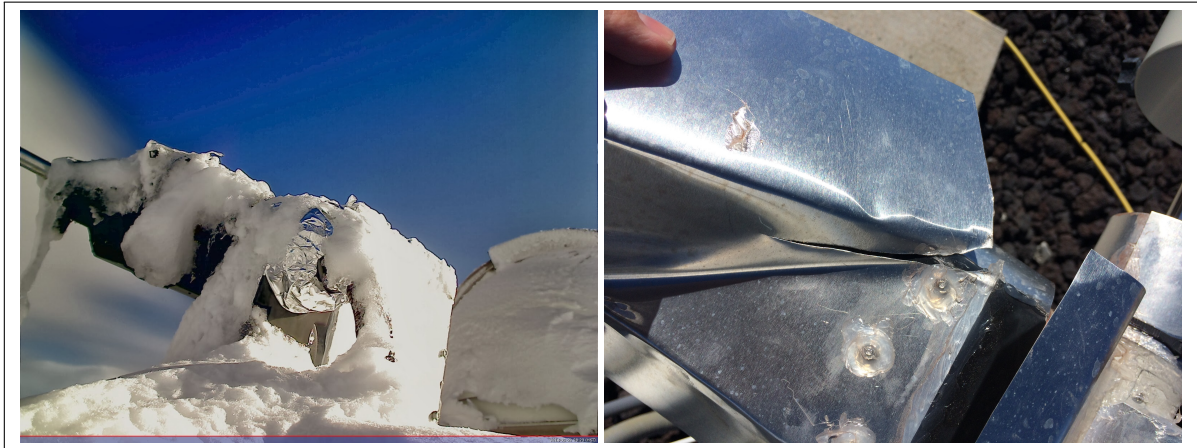
Figure 1.7: Left: PANOPTES prototype happily parking through the occasional Hawaiian blizzard. Image by Olivier Guyon. Right: Tearing of sheet metal due to high winds. Sheet metal designed to divert rain from joint interactions is shown after nearly six hours of sustained high winds ( \sim 150 kph). Weatherproofing worked effectively for nearly two years before tear occurred. Image by Josh Walawender.
