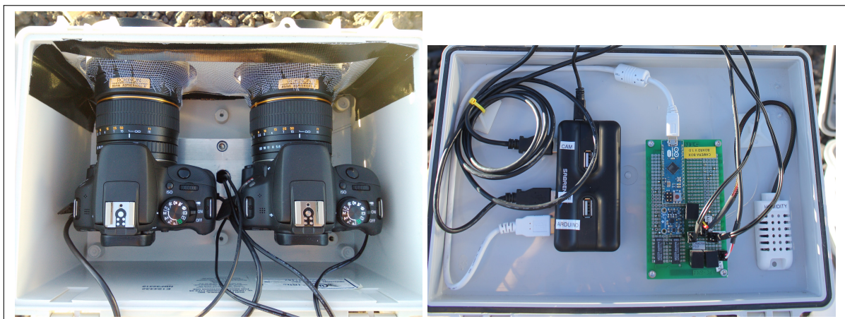
Figure 3.2: Images showing inside of camera box. Left: The two DSLR cameras mounted on top of the internal aluminum plates. Power and USB cables are seen entering through the center of the aluminum plates. Right: A USB hub and the camera electronics board are attached to the lid of the camera box. A temperature/humidity sensor and a 9-axis accelerometer are also visible.
