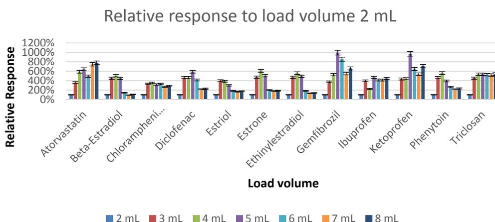
**Figure 3.21 :** Relative responses compared to responses at 2 mL min<sup>-1</sup> obtained under run conditions ACN/water carrier; negative ESI mode. Error is estimated from precision experiments (Section 3.1.7)
