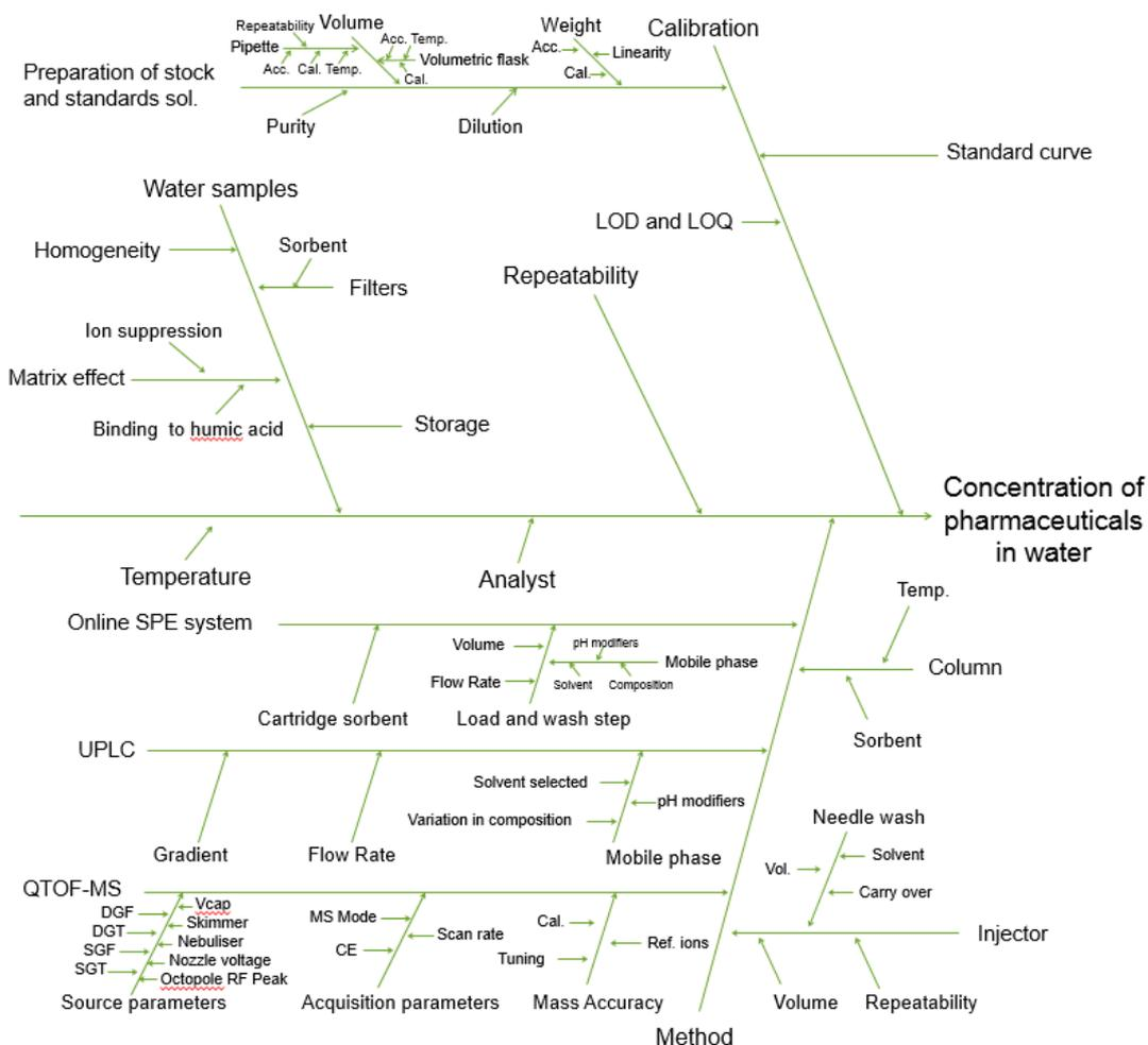
**Figure 3.1 : Ishikawa diagram identifying causal factors that contribute to the desired outcome of a method for determining the concentrations of pharmaceuticals in water**
