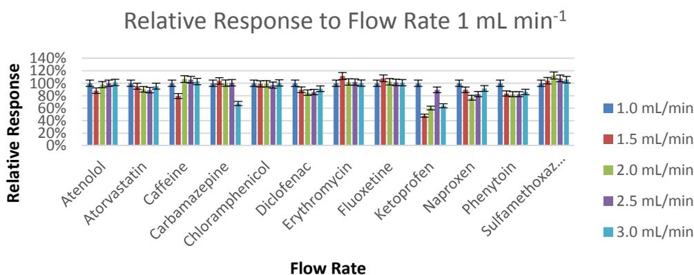
**Figure 3.20 :** Relative responses compared to the responses at flow rate of 1 mL min<sup>-1</sup> under run conditions ACN/0.1% formic acid carrier; positive ESI mode. Error is estimated from precision experiments (Section 3.1.7)
