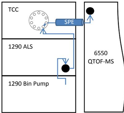
**Appendix 9 : Schematic for SPE-UHPLC-QTOF with a. load position and; b. elute position**
