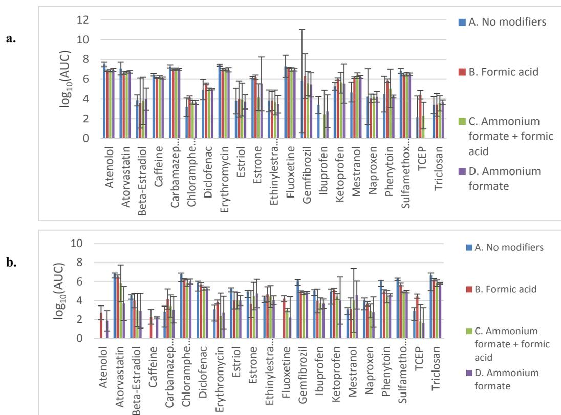
**Figure 3.4 : Comparison of the  $\log_{10}(\text{AUC})$  of each compound against the four chromatographic buffer conditions for a. positive ESI mode and; b. negative ESI mode.**
