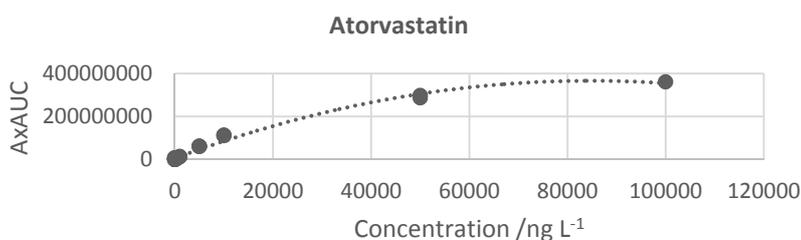
**Figure 3.23 : Calibration plot of atorvastatin, with response plateauing at higher concentrations.**
