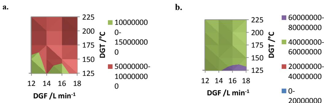
**Figure 3.8 :** Surface charts of responses from different combinations of DGF and DGT values acquired in ACN/water mobile phase in a. positive ESI mode and; b. negative ESI mode. The different shades represent the total response of the compounds.
