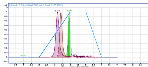
**Figure 3.15 : Chromatogram of the three compound mix, with caffeine at 3.163 min (purple), sulfamethoxazole at 3.4 min (brown), and ketoprofen at 3.930 min (green). The binary gradient is represented by the blue line, where it starts at 5% and steps up to 95% below returning to starting conditions.**
