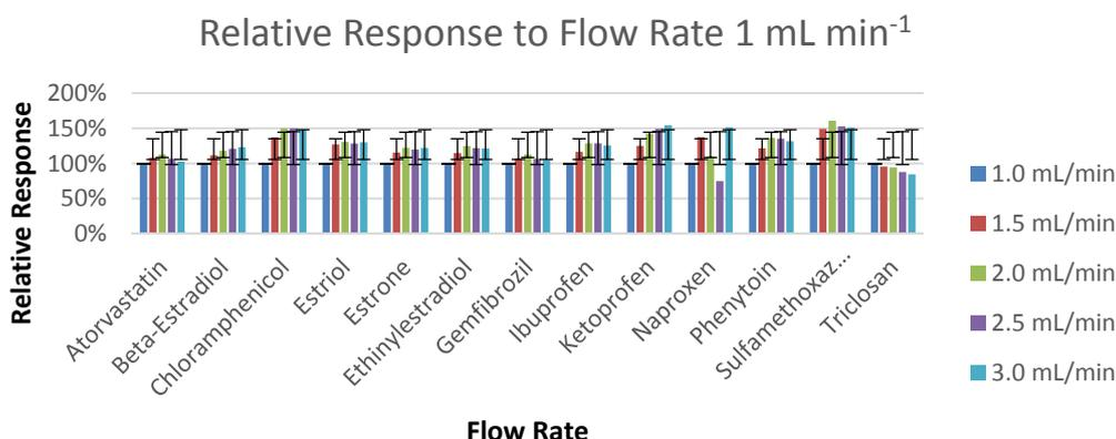
Figure 3.19 : Relative responses compared to the responses at flow rate of 1 mL min<sup>-1</sup> under run conditions ACN/water carrier; negative ESI mode. Error is estimated from precision experiments (Section 3.1.7)
