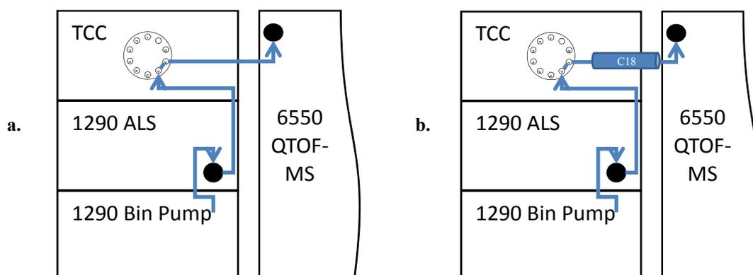
**Figure 3.3 : UHPLC-QTOF-MS schematic for a. flow injection with column bypass and; b. chromatographic analysis with C-18 column.**
