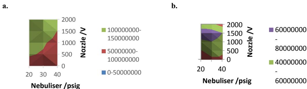
**Figure 3.6 : Surface charts of responses from different combinations of nebuliser and nozzle values acquired in ACN/water mobile phase in a. positive ESI mode and; b. negative ESI mode. The different shades represent the total response of the compounds.**
