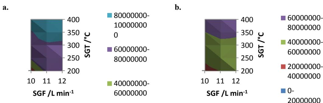
**Figure 3.7 : Surface charts of responses from different combinations of SGF and SGT values acquired in ACN/water mobile phase in a. positive ESI mode and; b. negative ESI mode. The different shades represent the total response of the compounds.**
