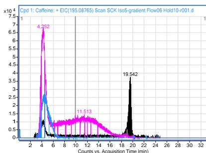
**Figure 3.13 : Overlay of the EICs where an isocratic 5% ACN:water is applied from 0-18 minutes, followed by an ACN clean up. Caffeine (blue) and sulfamethoxazole (pink) have eluted at isocratic conditions, whilst ketoprofen (black) only elutes when a high ACN content is applied.**
