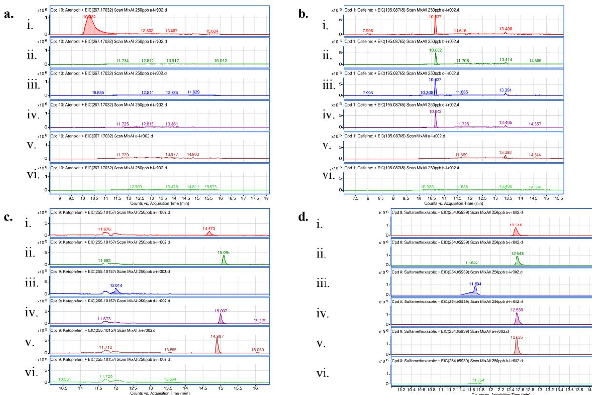
**Figure 3.17 : EICs of compounds at different load conditions (i-vi corresponding to conditions in Table 3.14) for a. Atenolol; b. Caffeine; c. Ketoprofen and d; Sulfamethoxazole**
