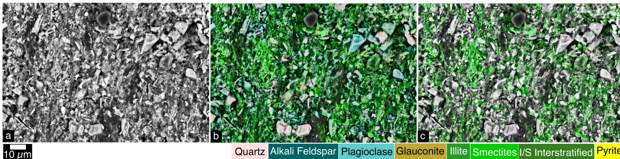
Fig. 2.6. SEM photomicrograph and Nanomin mineral maps of a Monterey Formation sample (M28). a: Backscatter SEM photomicrograph showing the majority of organic matter is present in an intimate association with clay minerals. In rare occasions, discrete, particulate organic matter is observed (top middle side of the image). Majority of these discrete organic particles in Monterey samples are possibly migrated, early-generated bitumen as indicated by their rounded shape, homogenous appearance and pore-filling nature. b: Bulk mineralogy of the same view as Fig. a. Feldspars (blue), Clay (smectites and illite) (green) and quartz (grey) are the dominating minerals. c: Nanomin mineral map for smectite and mixed layer illite-smectite of the same view as Fig. a and b. Amorphous organic matter (black patches) is intimately mixed with smectite and mixed layer illite-smectite. Submicron size smectite and illite-smectite flakes are spotted within organic matter.
