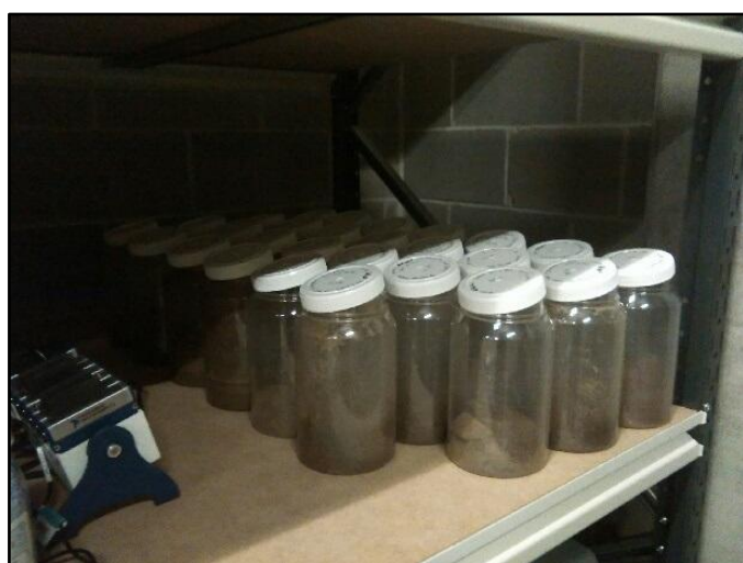
Fig 7. Pots as stored during the experimental phase. Lids are askew so as to allow for escape of GEM. Light is artificial. After each weekly sampling, vessel placement was randomised. The setup is indicated on the right
