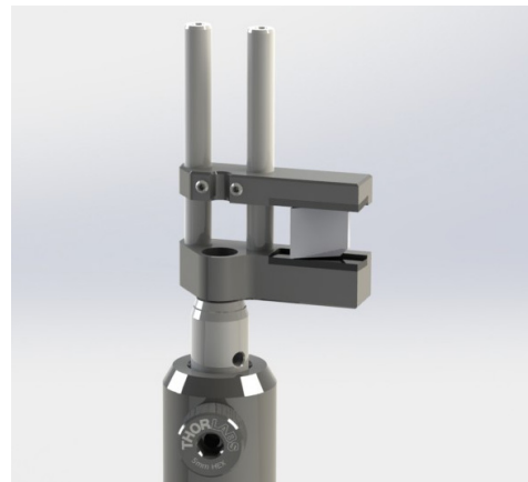
(d) The PS873-A prism operates over a wavelength range of 350-700 nm and has an apex angle of 30^\circ . It's made of N-KZFS8 with a refractive index of 1.7249 @ 550nm.
