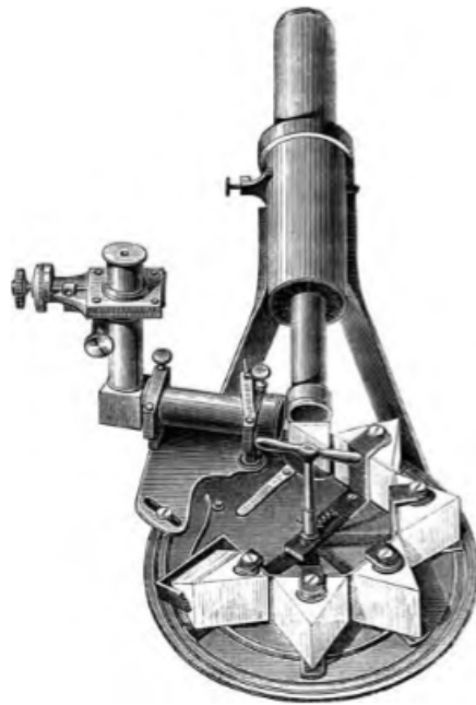
Figure 1.7: Angelo Secchi's multi-prism, double-pass spectrograph. (Hearnshaw, 2009)
