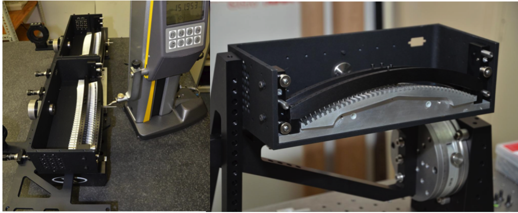
Figure 2.7: Curved slit assemblies on the translation stage of HERMES. This allows the light from the 2 sets of 400 fibres to be correctly injected and exchanged, increasing observational efficiency (Sheinis et al., 2015).
