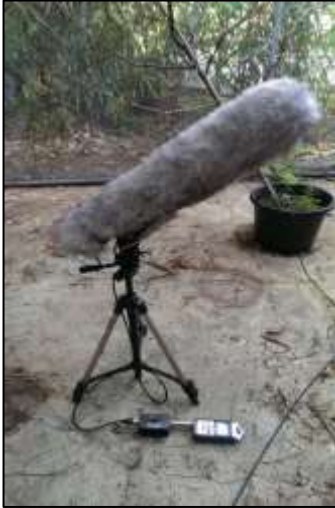
Figure 3. Regent honeyeater ( Anthochaera phrygia ) pre-release enclosure equipment set up. Sennheiser directional microphone fitted with windshield and 48V phantom power supply connected to Zoom (4Hn) handheld recorder.
