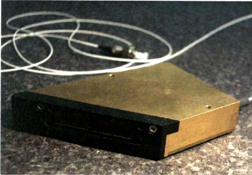
FIGURE 4.1: Top: schematic of the AWG chip. Bottom: photograph of the IPS prototype. In this prototype device (Chipset A), the output array waveguides (standard in commercial devices) have been removed, the output facet has been polished back to the focal surface, and the chip packaged. The fibre input is at the rear of the image, and the polished flat output facet at the front. The open face of the chip is \sim 38 mm in length. The active area is \sim 3 mm across, and is situated at the centre of the polished face.
