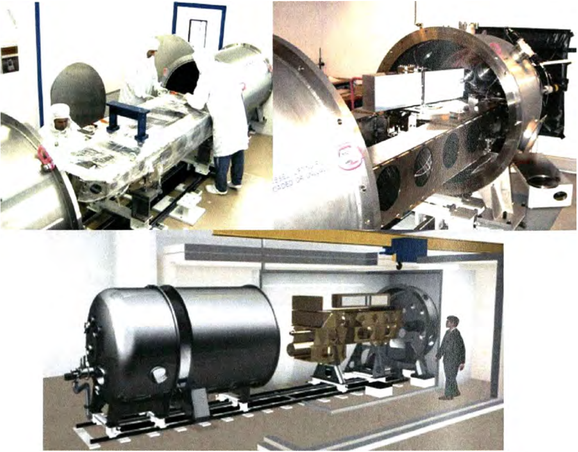
FIGURE 6.10: A series of images taken during the construction of the HARPS high resolution spectrograph (top left and top right), with a CAD image showing the overall size of the spectrograph (bottom). These images illustrate the relative scale of the spectrograph itself, the large Echelle grating based on a mosaic construction, and the vacuum chamber. Images courtesy of Lovis et al. [107].
