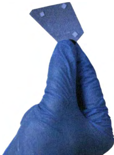
FIGURE 4.17: Image showing the Chipset B AWG. Chipset B has no input waveguide/fibre and no protection housing.
