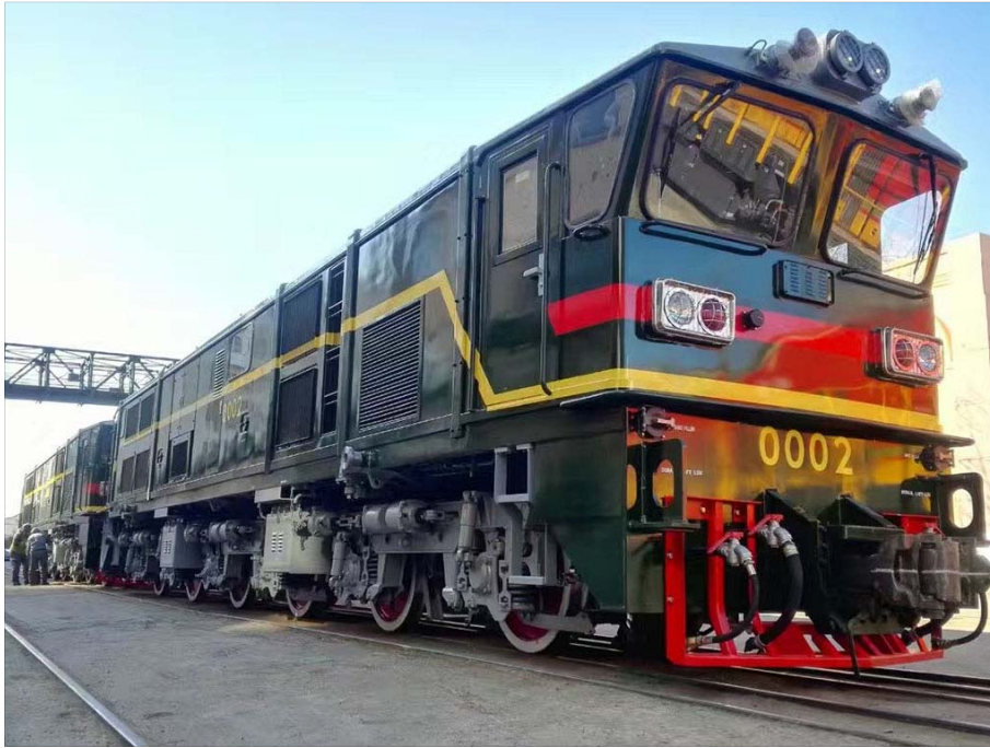
Plate 11: A Type CKD7B design Bo-Bo-Bo locomotive, manufactured by CRRC Dalian of China.
