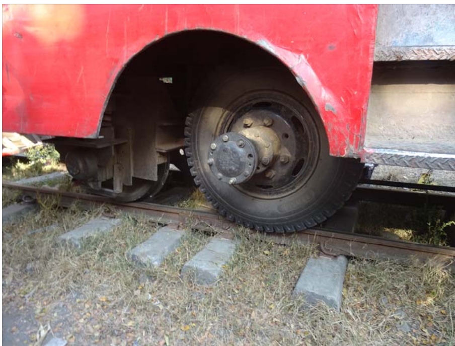
Plate 24: The rubber tyre on a wheel on an axle, providing power to move the LRBE along the track.
