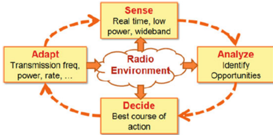
Figure 2.2: Functional Architecture of a Cognitive Radio
